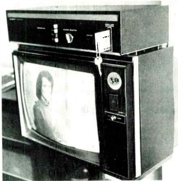
Key code. Plastic key unlocks control box in Telebeam system for room security, pay-TV, and hotel management.
