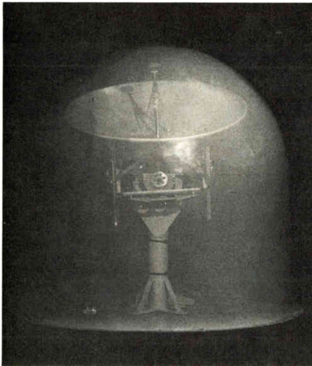
2. Under the dome. The Marisat shipboard terminal being built for Comsat General by Scientific Atlanta has a 4-foot antenna and uses a low-noise transistor amplifier. The platform, which is stabilized for pitch and roll, is covered with a fiberglass radome.
