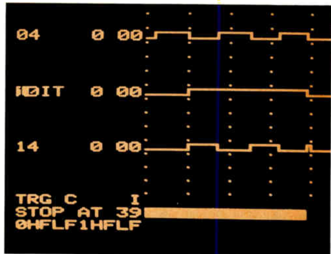
6. Capture. Glitch on trace 14 occurs at the trigger point denoted by end of trigger delay bar at screen bottom. This, teamed with transitions on other channels, could cause a system malfunction.
