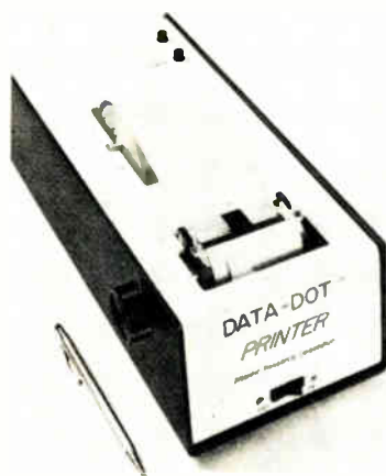
Dot's right. White square on TV screen shows relative area to be occupied by Data-Dot. Thermal printer will decode data and print out message transmitted with the TV picture.
