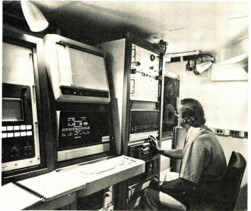
Tracker. RCA technician Charles Peterson checks out computer control of Digital Instrumentation Radar. Housed in mobile shelter, system will be used on test ranges.
