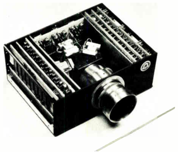
Ring around a prism. Bell Labs' CCD color camera of the Picturephone type has three CCD chips arranged around a prism to form the color images. Several other devices have been made using the three-level polysilicon approach.
