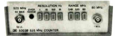
5303B — 525 MHz Counter Module: DC to 525 MHz range, burst or CW frequency. 50Ω or 1 MΩ input. Automatic gain control. Fuse protected front end. Optional high stability time base (FCC Type-Approved). $800.
