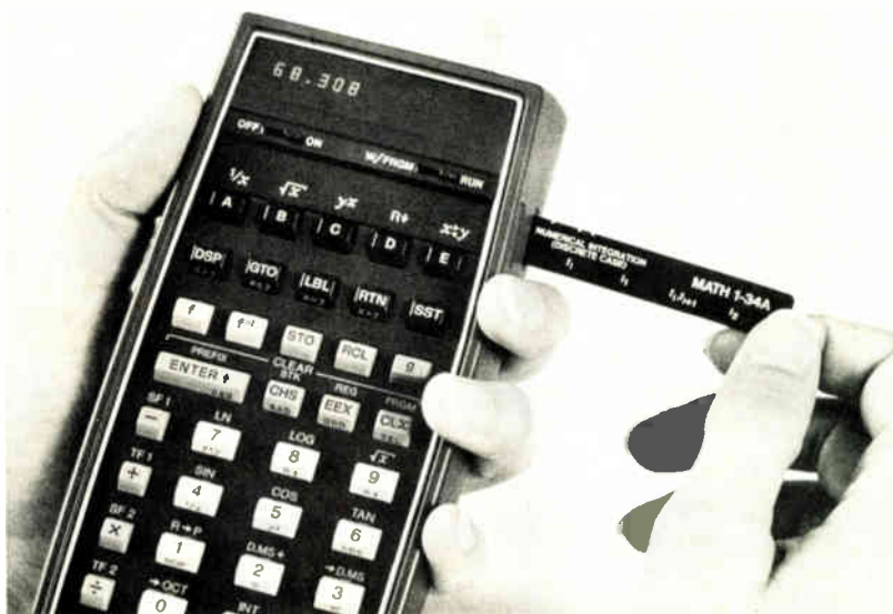
Engineer's assistant. Photo at left shows HP-65 being used to figure sidewall capacitance; right photo demonstrates method in which the magnetic program card is inserted.
