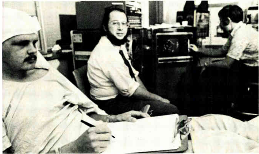
Patterns. A blind patient can draw patterns displayed on a CRT shown at the rear and sent to his brain via electrodes implanted in his visual cortex. A DEC GT Graphics-40 System controls the setup. Associate director of the project is William Dobelle (center).
