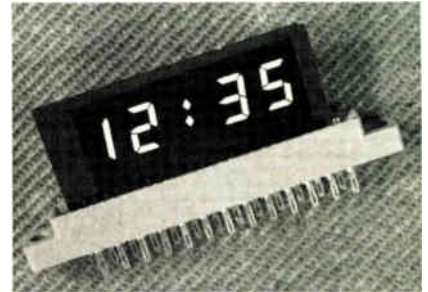
From New Jersey. This is electrochromic display produced by the Optel Corp.
