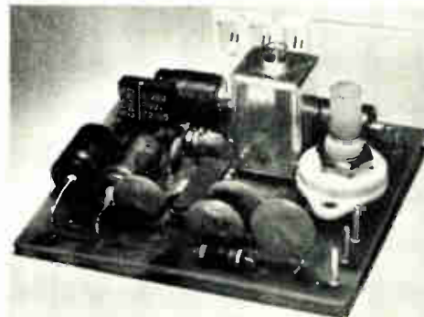
Deflection and sound. On board at left is TDA 1170, an IC that performs functions of vertical-deflection system. On board below is the 1190, a complete audio channel.
