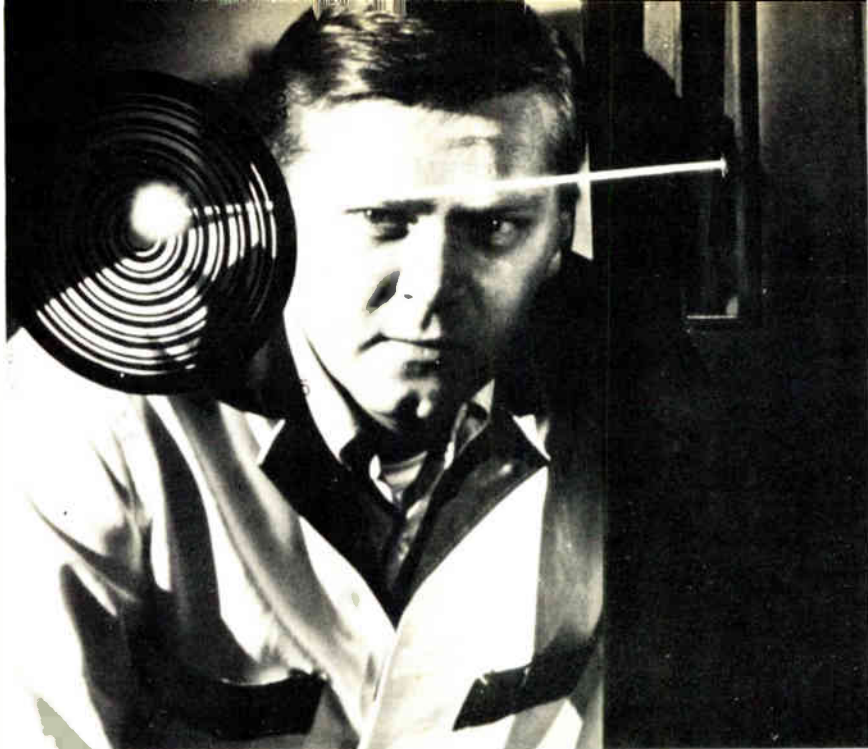
Laser baggage sorter. Automatic label-reading device developed by Bendix senses codes that define flight numbers and destinations. This system will be used at Miami airport.
