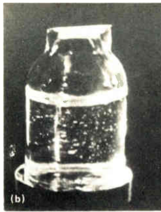
4. Keep It clean. Video image differentiator checks transparent pharmaceutical preparations for visible impurities (a). By subtracting the TV image of the bottle containing moving particles (b) from a second image of the same bottle, the nonmoving background is deleted (c).
