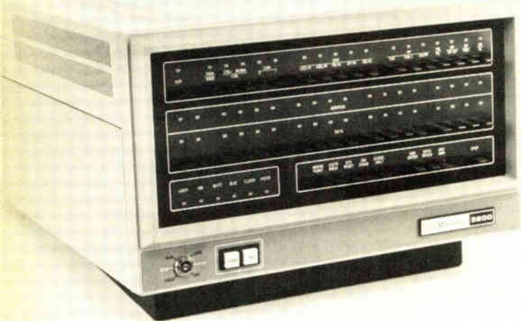
5. Microdata 3200. New minicomputer uses firmware-controlled stack concept to run efficiently on PL/1-like high-level language.
