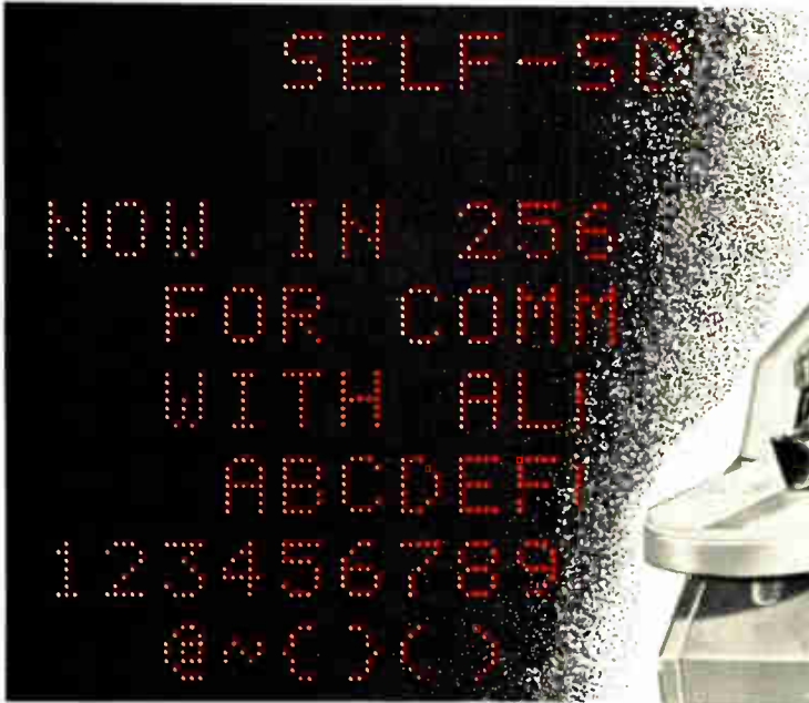
SELF-SCAN Panel Display Subsystem, 256 Character Capacity, 5 x 7 Dot Matrix. Characters 0.25" High. 64-character format, available with all drive electronics including memory, character generator, and timing.
