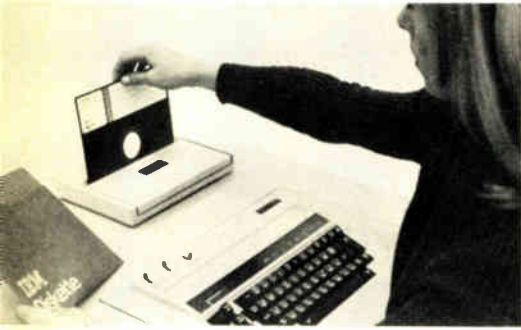
Data entry. IBM's 3740 system performs the same job as punched cards, but it's faster.
