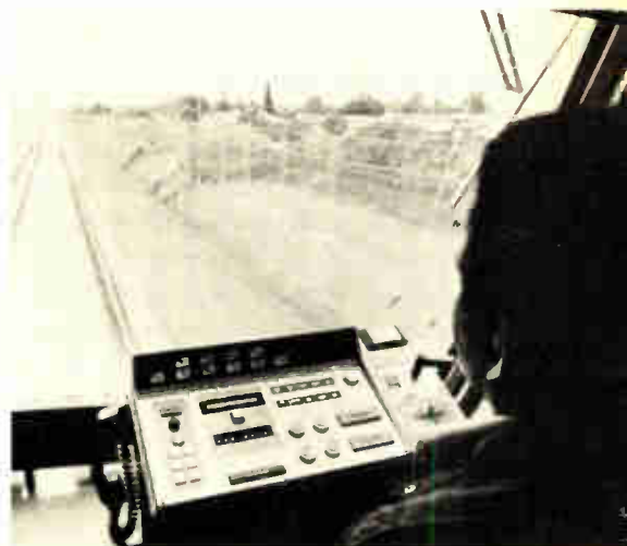
Hands off. View from the front end of a BART car shows Westinghouse controls.
