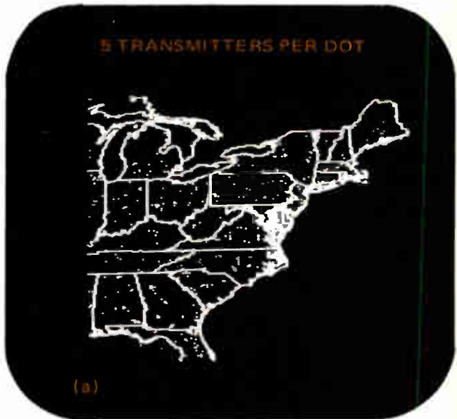
10. Equipment density. By accessing ECAC's extensive files, a CRT terminal can obtain a map of the density of radio transmitters assigned within specified band limits. Progressively smaller geographic regions can be requested until ultimately a printout of each station in the data bank is identified by equipment characteristics.
