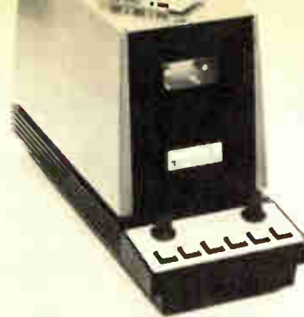
12. Cassette drive. Two Philips cassettes can be used on this drive to provide a million bytes of low-cost sequential mass storage.
