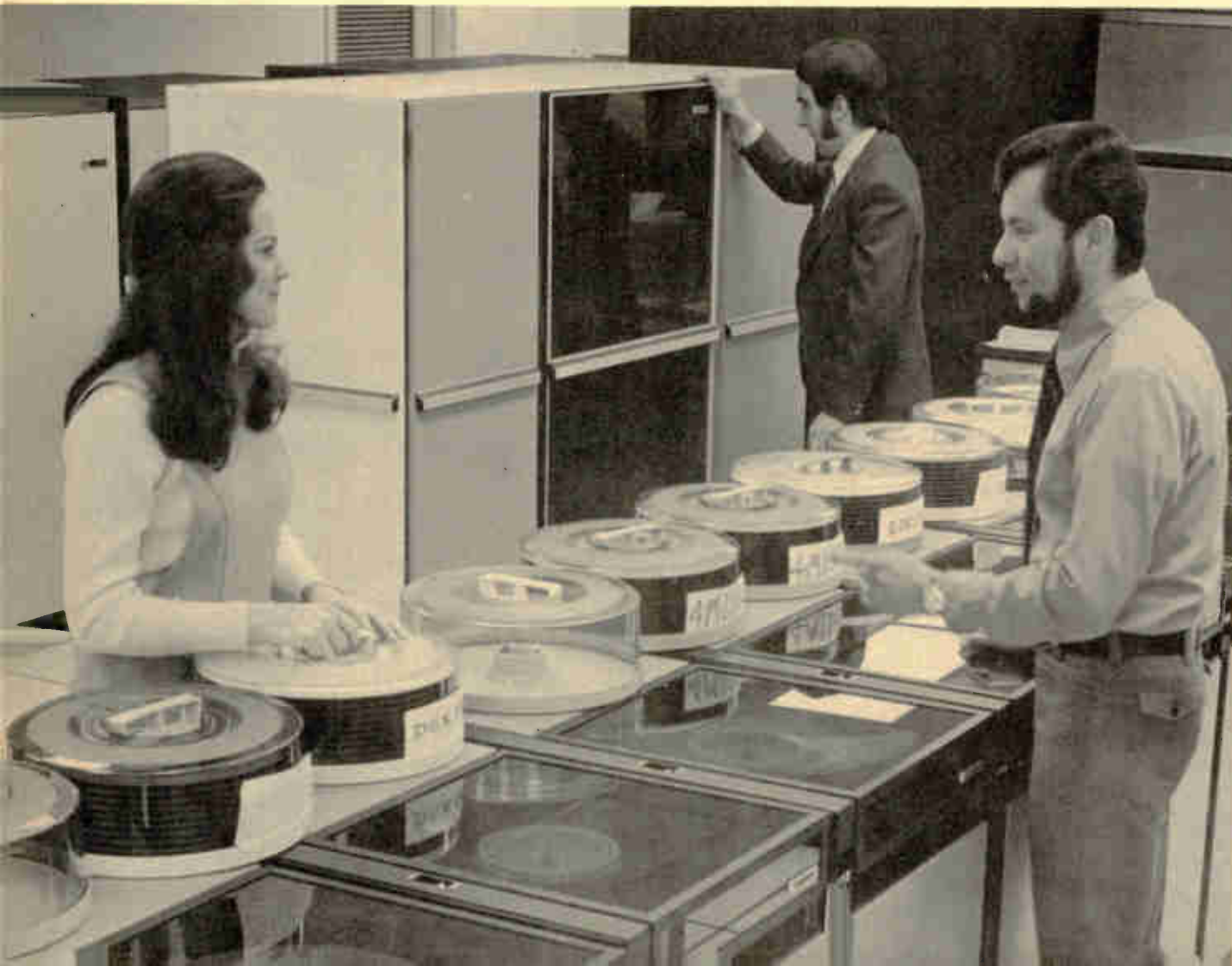
13. Disk-pack units. Ampex DS-314 disk storage units use interchangeable packs, each capable of storing up to 29 million bytes.
