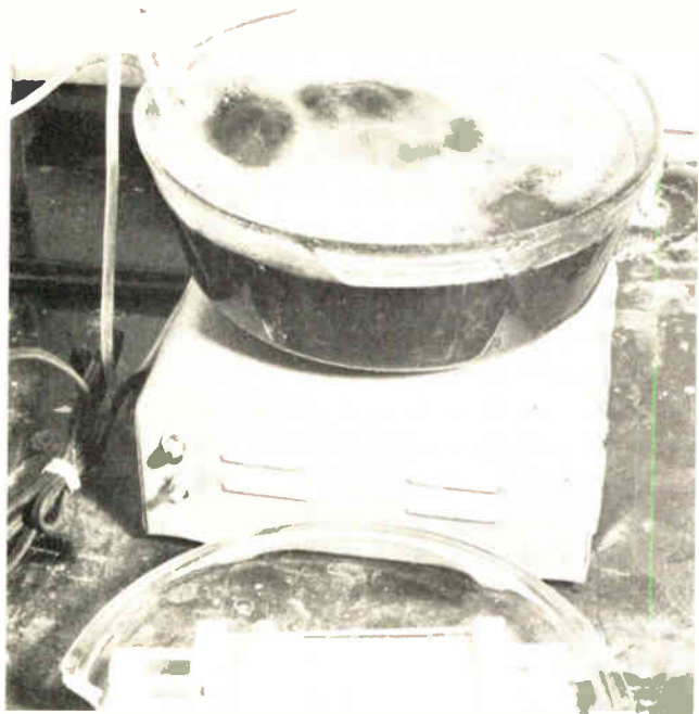
The continuous air flow through the aerators creates a surface froth that scrubs the board with constantly agitated etchant. The sliding clamp holder which is attached to the cover dish permits rapid insertion or reversal of the printed-circuit board.
