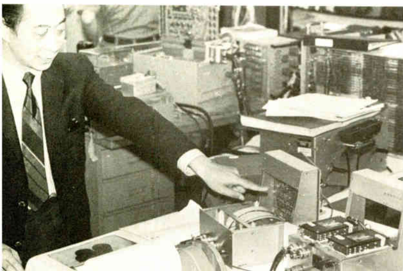
1. Small and simple. Author Chung points at some prototype T-boxes on a bench at United Technology Labs. The boxes plus computer software replace large, expensive input-output controllers.
