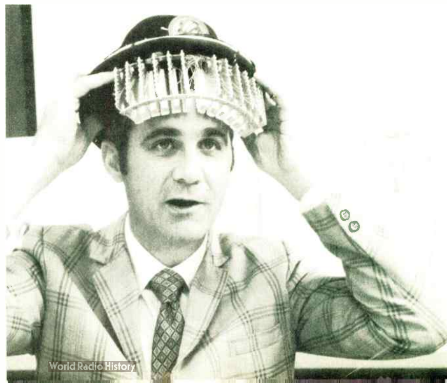
Boll: Torsovision for 20,000 to 30,000 blind as light is converted to bursts of air.
