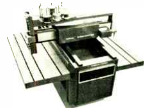
Semi-automatic wire terminating and harness laying equipment (RS 296)
