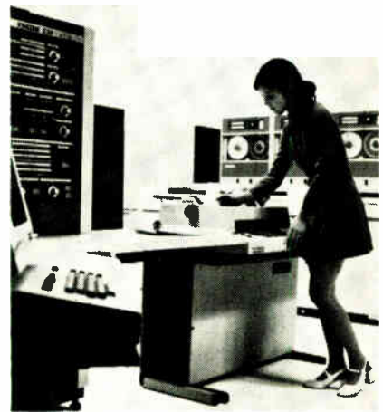
To the wire. Two models in Fujitsu's new computer line-up feature plated-wire memories, one of which boasts a 1-million-word capacity.
