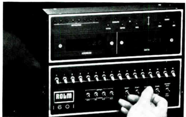
7. In control. The control panel uses light-emitting diodes for address and data display. The module is in a separate housing from the central processor and memory unit, allowing remote operation in aircraft or industrial jobs.
