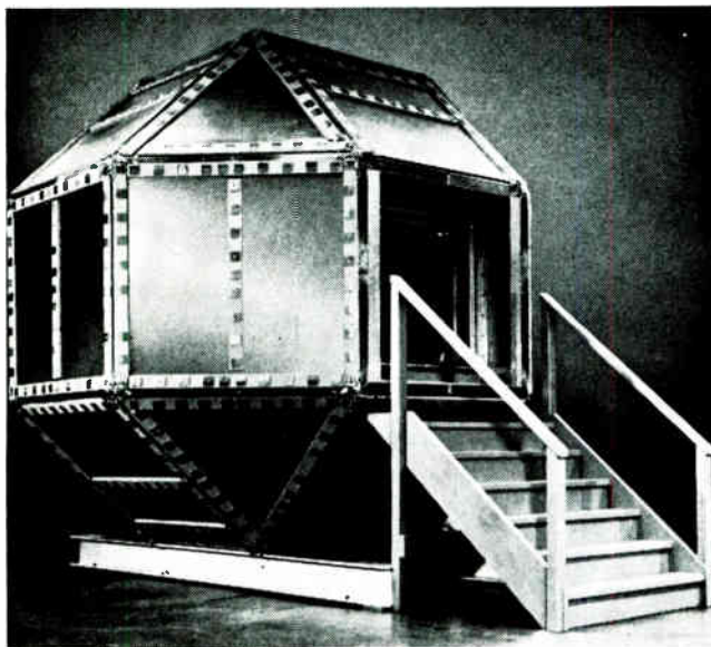
1. Cardiograms with Josephson junctions. At MIT, magnetometer built with Josephson junctions measures body's magnetic field. Resulting magnetocardiograms, like the one shown, may contain more information than electrocardiograms. Since changes in body's field are small, room in which measurements are taken has to be shielded against changes in the earth's magnetic field.
