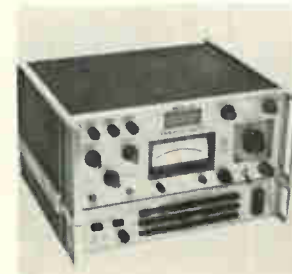
Tunable, lock-in voltmeter is for a wide range of low-level signal and noise measurement. The instrument is made up of a combination of the company's standard model 132 lock-in signal-to-noise meter and the new model 500 programmer with tunable frequency range from 1 hz to 1 khz. Brower Laboratories Inc., 237 Riverview Ave., Newton, Mass. 02154 [368]
