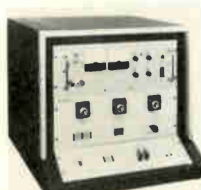
Nondestructive tester model 33 measures the safe operating region of power transistors. Power supplies with various voltage and current ratings are available. Extremes of the available ranges are 60 v at 30 amps and 330 v at 4 amps. Test time can be varied by a front panel control from 10 msec to 10 sec. Test Equipment Corp., 2925 Merrell Rd., Dallas 75220 [366]
