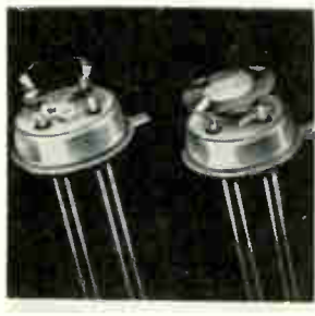
Crystal controlled IC oscillator model MCO-F, which uses thin-film capacitors and resistors on a single substrate, is totally contained within a 4-lead TO-5 Koldweld package. Operating in the 5 Mhz to 25 Mhz frequency range, it offers a frequency stability of \pm 0.003\% from -55^{\circ} to +125^{\circ}\text{C} . TRW Semiconductor Division, 14520 Aviation Blvd., Lawndale, Calif. 90260 [343]
