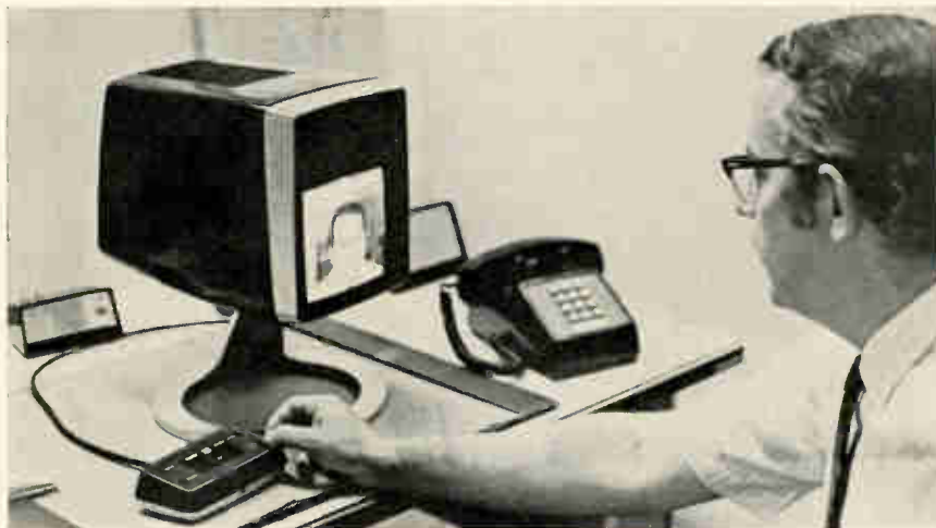
Getting the picture. Here's a typical Picturephone installation in Pittsburgh. That's the control box at left, speaker behind it.
