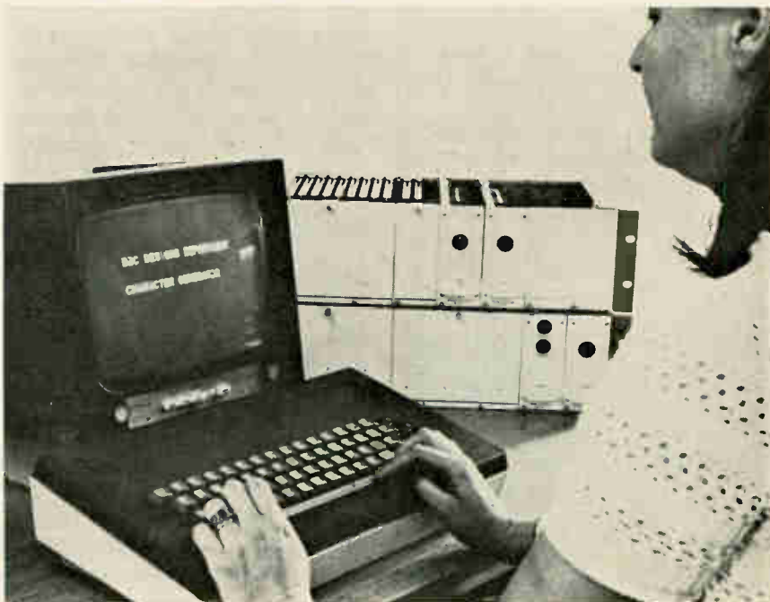
At the keyboard. The Anchor system accepts commands for generating a character from a computer, from a paper tape reader, or from a keyboard. Overall cost is no more than for dot matrix generators, developers say.
