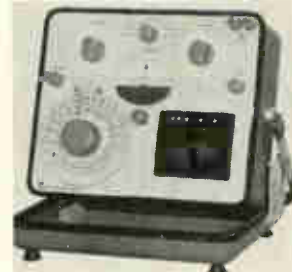
Impedance bridge model 1656 features 0.1% basic accuracy, ease of balance, portability and low cost. Lever arm switches permit fast balances and easy-to-read answers for measurements of C, L, R, and G. Unit also measures D and Q, using a dial indicating technique. A 1-khz generator is included. Price is $700. General Radio Co., West Concord, Mass. 01731 [364]
