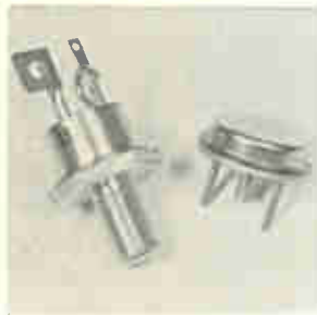
Planar epitaxial, pnp power transistors are available up to 100 amps. The SDT3600 comes in the TO-68 case, and the SDT 3900 in the TO-114 case. Features include 50 amp saturation voltage less than 1.5; h_{FE} at 90 amps, 10 typically; less than 10 \mu a leakage currents; on and off times less than 2 \mu sec at 100 amps. Solitron Devices Inc., Riviera Beach, Fla. [437]
