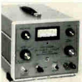
R-f power leveler model 1805 ensures precision in systems used for transferring calibration factors of primary standards to bolometer standards or secondary power standards and power meters. It has minimum power level control range of 20 db and employs only d-c substituted and bias power to maintain precise power levels. Weinschel Engineering, Gaithersburg, Md. [407]
