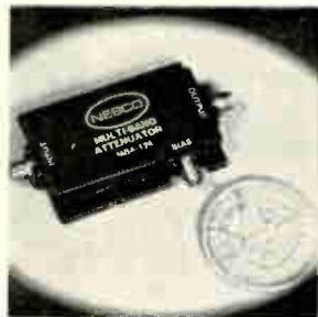
Multiband variable attenuator MBA-124 can handle all signals in the uhf, L, S, C, and X bands with a flat response and a very low insertion loss. Unit is flat to \pm 4 db deviation between 0.5 Ghz and 12.4 Ghz for any value of attenuation down to a minimum of 60 db isolation. The compact device will handle 1 watt of c-w power. Nesco Mfg. Co., 28 Osgood St., Methuen, Mass. [402]
