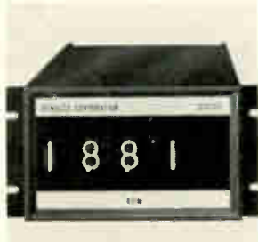
Digital tachometer series D9000 displays rpm directly, or any other rate information such as gallons per minute, inches per second, etc. Signal inputs may be obtained from magnetic pickups, photocells, contact closures or shaft encoders, with any number of pulses per revolution or frequency range. Price is $354. Dynalco Corp., 4107 N.E. 6th Ave., Ft. Lauderdale, Fla. [362]
