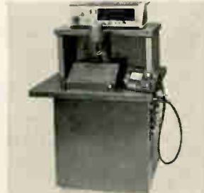
Laser system model SS-218 is used for trimming thick and thin film resistors, capacitors, and other deposited materials. Units, which operate at a variety of pulse repetition rates and energy levels, are completely shielded for operator safety. Resistor trimming accuracy is better than 0.1% over a range of 1 ohm to 11 megohms. Raytheon Co., Waltham, Mass. 02154 [427]
