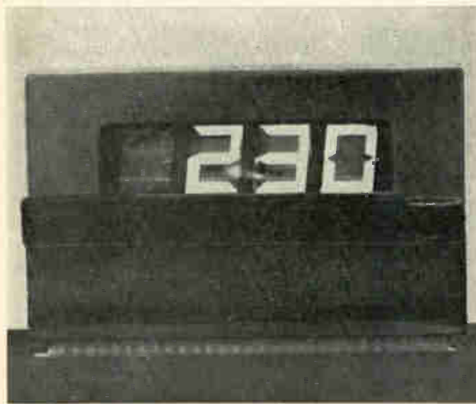
In good time. Electronic clocks with liquid crystal numeric indicators may soon be here. Each numeric panel consists of a glass/liquid crystal/glass sandwich with segmented electrodes etched on one glass plate by photoresist techniques. Flat structure could be adapted to battery-operated wristwatches.
