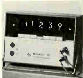
Digital multimeter UGWD is a compact set for measuring d-c and a-c voltages from 100 \mu v to 1,000 v and resistances from 1 ohm to 15 megohms. The stored display gives an accurate three-digit readout with a fourth digit of "1" for overrange indication. Unit can be used in the lab and production. Rohde & Schwarz Sales Co., 111 Livingston Ave., Passaic, N.J. [363]
