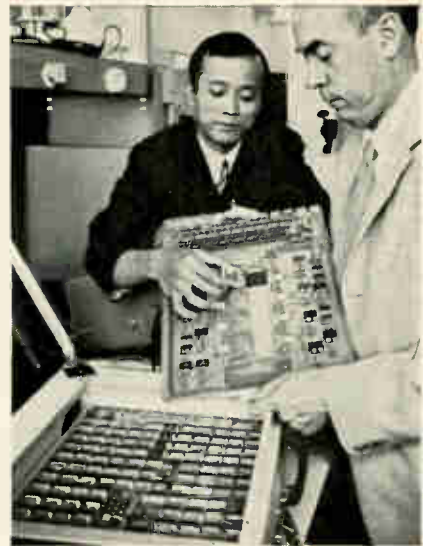
Building blocks. Cofelec's ROM is built up of snap-out modules.
