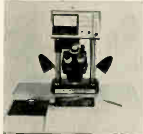
Manual die bonder model HDB-900 is a self-contained unit that utilizes the eutectic method for bonding semiconductor chips to substrates or headers. It features a work chuck that is a separable but interchangeable part of the heated stage, providing simple change of chucks for hybrids or semiconductors. Hughes Welders, 2020 Oceanside Blvd., Oceanside, Calif. [426]
