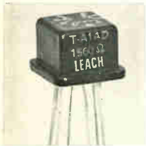
Microminiature relay series T is for high isolation switching and r-f use. The 2 pdt unit is rated at dry circuit through 1 amp resistive, operates from -65^{\circ} to +125^{\circ}\text{C} , and has a life at rated load of 100,000 cycles. Contact bounce is at a low 0.0015 sec maximum, and the unit has a dielectric strength at sea level of 500 v rms. Leach Corp., 5915 Avalon Blvd., Los Angeles [341]
