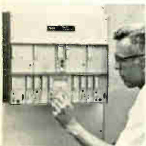
R-f repeater FR2000 for point-to-point systems, makes use of microwave IC-type amplifiers to provide 90 db of gain at 2 Ghz. It can be used to reduce the costs of new routes, to replace out-dated heterodyne repeaters, or to eliminate path problems on existing routes. It is small in size and consumes 35 w of power. Farinon Electric, 935 Washington St., San Carlos, Calif. [405]
