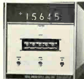
Digital synchro display model 1841 accepts two-speed (1:1 and 36:1) synchro position information and provides 5-digit angle display. It is all solid state and uses no rotating mechanisms or optical devices. Two display ranges, 0 to 360° and 0 to \pm 180°, with the same zero reference provide added flexibility. Price is $2,400. Scientific-Atlanta Inc., Box 13654, Atlanta, Ga. [367]
