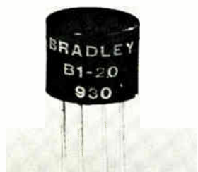
Encapsulated silicon bridge rectifiers series B1 are rated at 1.5 amps and are available in voltage ratings of 50 to 1,000 piv. They are intended for rapid insertion into p-c boards. Units save the user the time and expense of selecting and matching individual diodes for piv, forward voltage drop, and leakage current. Bradley Semiconductor Corp., 275 Welton St., New Haven, Conn. [441]
