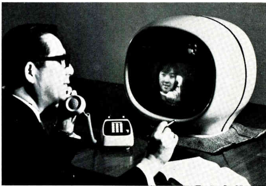
Seeing double. Standard 12-inch color tube is used in Toshiba's colorphone for seeing caller; a 3-inch black and white tube monitors outgoing image.
