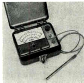
R-f voltmeter model 500 covers the frequency range from 20 khz to 500 Mhz with a voltage range from 200 mv to 15 v rms. From 20 khz to 100 Mhz, measurements are accurate to 3% of full scale; from 100 to 200 Mhz, accuracy is 5%; and from 200 to 50 Mhz, voltages are read from a calibration curve. High Frequency Engineering Co., 2626 Frontage Rd., Mountain View, Calif. [367]
