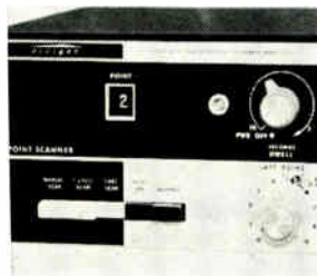
Ten point scanner model 634 is used to sequentially transfer analog data from multiple sources to one measuring instrument. Scanning is accomplished by two-pole reed relays suitable for switching low level sources, such as thermocouples. Dwell time on each point is adjustable by front panel control. Price is $575. United Systems Corp., 918 Woodley Rd., Dayton, Ohio 45403 [362]
