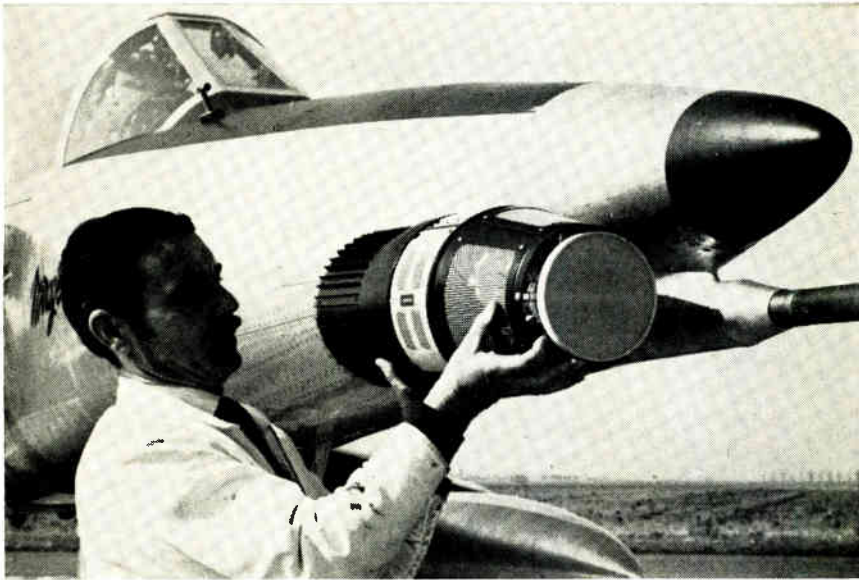
Leitmotiv. The light weight and small size of the Aida-2 fire-control radar allow easy fit in nose cone of Mirage or other light interceptors.
