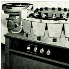
Transistor sorter type 1635 was developed to automatically test and sort TO-105 and TO-106 epoxy type transistors at a rate of 5,000 or more per hour. It automatically feeds components from a vibratory bowl via an orienting track to a 16-station index table which advances them to either a single or dual test probe. Daymarc Corp., 40 Bear Hill Rd., Waltham, Mass. [425]
