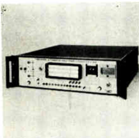
Automatic diode classifier type D189 can test over 10,000 diodes an hour, making all standard tests and assigning devices to as many as 8 different categories. It measures reverse voltage to 1,200 v in 2 ranges and can deliver up to 10 amps for forward-voltage tests. Reverse-leakage-current range is 0.005 to 1,000 µa. Price is $13,500. Teradyne Inc., 183 Essex St., Boston. [365]
