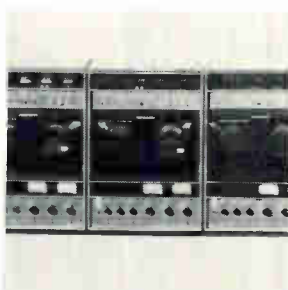
Automatic plasma machine IPC 2003 is designed for wafer stripping and photoresist removal. It contains two 3-x-6-in. plasma reactors, and a single reactor window covers both reactors. It has three automatic cycles, each of which can be set at 0-300 watts, 0-900 cc per minute gas flow, and 0-99 minutes. Monte Tool Associates, 25222 Cypress St., Hayward, Calif. [427]
