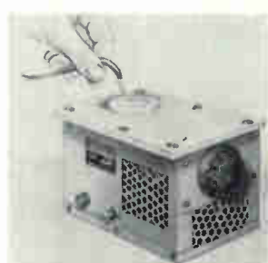
High-temperature (in excess of 1,300°F) silver soldering pot eliminates need for chemical or abrasive removal of film insulation and use of soft solder and soldering iron when joining magnet wires to leads. Dipping wires into molten solder simultaneously strips insulation and encases them in a permanent silver solder coating. Precision Electronics Corp., Marshfield, Mass. [428]
