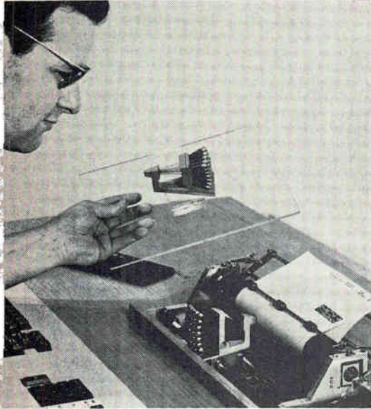
Type cast. An array of solenoids at one end of type head push pins at other end to generate characters.
