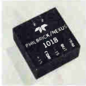
Chopperless, differential operational amplifier model 1018 features low drift. It employs dual-input transistors with a precision metal-film resistor and a bias current compensation network. This results in high thermal stability and low static offsets. Typical gain is 2,000,000; output, \pm 3.5 ma at \pm 13 v. Philbrick/Nexus Research, Allied Dr. at Route 128, Dedham, Mass. [382]
