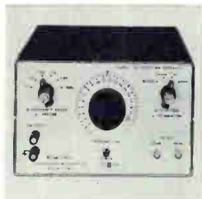
Function generator model 743 provides low distortion sine, square, and triangular waves over a dial-controllable range reaching 2 megahertz, with an output of up to 20 v p-p from a 50-ohm source impedance. In the frequency-modulation mode it is possible to sweep from 1 hz to 4 Mhz. Clark-Hess Communication Research Corp., 43 W. 16th St., New York 10011 [362]
