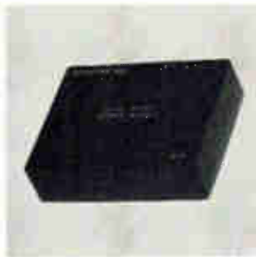
Encapsulated power supply model 527 provides two 15 v power supplies capable of common external connections with an accuracy of 1%. Each separately regulated supply provides a full 50 ma of output current. Output regulation, line or load is \pm 0.2\% . Temperature stability is \pm 0.02\% / ^\circ\text{C} . Price is $39; delivery, stock to four weeks. Burr-Brown Research Corp., Tucson [385]
