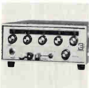
Variable d-c voltage standard model V-2000 features 1 \mu v resolution and 0.005% accuracy. Output range is up to \pm 11.1110 v in 5 decades. Front-mounted rotary switches control illuminated readout. A \pm 1 mv vernier switch aids range control. Output current of 50 ma increases versatility. Price is $625. Esterline Angus Division of Esterline Corp., Box 24000, Indianapolis 46224 [367]
