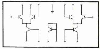
4. Improve your computer's memory with Linear Circut 5733. It's the video amplifier that operates over – are you ready? – 120 MHz band width! Differential in/differential out with minimal phase distortion, too. And as a pre-amp in computer applications, don't forget: 1) 10 ns rise time; 2) fixed gains of 10, 100, 400 available (variable between 10 and 400 with a single, external resistor); 3) internally compensated (no external frequency compensation components required.)
