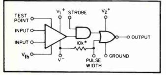
3. Improve your computer's memory with Linear Circuit 526 – the high-speed comparator that's beyond compare! (Do you know of another comparator with a propagation delay of 30 ns?) Other features to remember: 1) operates from  $\pm 5V$  supplies; 2) overdrive recovery, 20 ns; 3) fanout of 10; 4) high gain operation; 5) output compatible with DCL, DTL and TTL.
