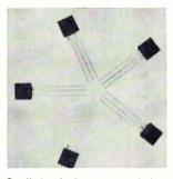
Small-signal TO-92 packaged plastic silicon transistors types MPSA10, MPSA20 (npn), and MPSA70 (pnp), are designed for low-level audio amplifiers and general purpose I-f amplifiers or switches in audio, radio, and tv circuits. They feature a breakdown voltage of 40 v minimum, low output capacitance of 4 pr max. Motorola Semiconductor Products Inc., Phoenix [438]
