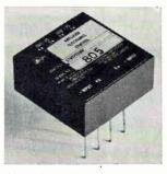
Four lightweight power amplifiers identified as the C70 3722 series are designed to drive either resistive or reactive loads in synchro driver or voltage follower applications. They meet the environmental requirements of MIL-E-5400. Rated output volts range from  $\pm 11$  to  $\pm 18.5$  v; rated output current, 135 to 500 ma. Singer-General Precision Inc., Little Falls, N.J. 07424 [388]
