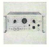
Preamplifier model 113 provides amplification of signals from d-c to 300 khz. Typical noise figures are 0.3 db maximum at 10 hz with a 2 megohm source impedance; 0.2 db maximum at 1 khz with a 1 megohm source impedance. Gain is from 10 to  $10^4$  in 1-2-5 sequence, continuously variable. Princeton Applied Research Corp., Box 565, Princeton, N.J. [387]
