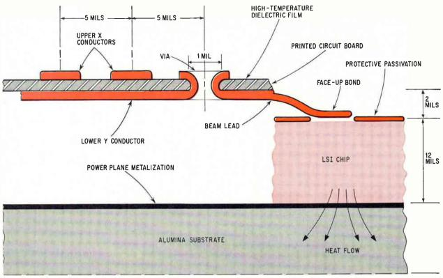
**Cross-section.** In one electroplating cycle, the beam leads are integrally formed with the upper and lower conductors and anchored by means of the vias. The beam lead, which contains a 2-mil offset for strain relief, is bonded face-up to the LSI chip. Thermal conductivity is through the alumina substrate base rather than the contacts. Power is delivered to the chip by a metalization layer on the substrate.
