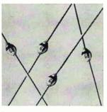
Axial lead fast recovery rectifier series A114 is for use in high frequency applications. It is rated at 1 amp in 50 to 600 v versions, with a 200 nsec maximum reverse recovery time. Unit has dual heat sink construction which provides rigid mechanical support for the pellet and excellent thermal characteristics. General Electric Co., 1 River Rd., Schenectady, N.Y. 13205 [443]
