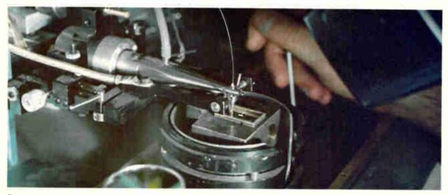
Bond watcher. Thermal monitor is designed to eliminate faulty IC-header bonds. The optical fiber, at center, extends from detector to bonder. Indicator lights tell if temperature level is too low to make a good bond, is just right, or is overheating chip.
