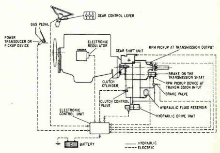
Look, no hands. Electronic control units, sensing transmission input and output speeds, takes over chore of shifting gears in heavy trucks.
