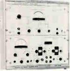
Bridge CB-154 Mark IV is for measuring capacitance, dissipation factor, and leakage current in electrolytic and tantalytic capacitors. Bridge-voltage supply is adjustable in 6 ranges between 1 mv and 3 v, with a choice of 60and 120-hz bridge frequencies and provision for external source up to 20 khz. Advanced Technology and Systems Corp., Riverside, Conn. [361]
