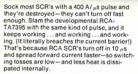
In addition to fast turn-off times, the TA7395 and other RCA SCR families have high dv/dt characteristics, and may be used at frequencies up to 25 kHz.
