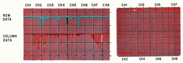
Analogs and digits. Multilevel analog pulses, top, built up in increments of -100 microamperes, represent dial or probe setting for each channel displayed on scope screen (right). With analog code, fewer connections are needed between plug-in and main frame than if binary digital code code were used.
