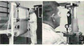
100% of all B-stage—in both rolls and sheet form—is visually inspected at Norplex to insure reliable, inclusionfree bonding sheets.
