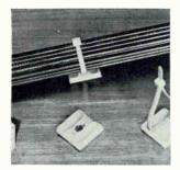
Adhesive backed mount ABMS-A secures wiring harnesses to virtually any smooth surface for light duty applications. Inclusion of a countersunk hole permits the mount to be used with a No. 6 flat-head screw or a ¼ in. flathead rivet. The result is a onehole mount which will not rotate. Mount measures 1¼ in. sq. Pandult Corp., 17301 Ridgeland Ave., Tinley Park, Ill. [345]
