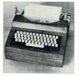
Input/output device for computers called Telewriter, measuring 13 x 18 x 7 in., and weighing 25 lbs, is interchangeable with the KSR33 Teletype. The printer input and keyboard output is serial 8 bit ASCII code. The Telewriter operates at a speed of 10 operations/sec (100 wpm). Electronic Information Systems Inc., Rural Route 3, Boulder, Colo. 80302 [425]
