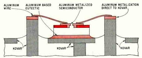
Nothing glitters. Gold, which is prone to catastrophic failure in harsh radiation environments, is replaced by aluminum in top posts, the lead wires bonded to those posts, transistor metalization itself, and eutectic bonding material. Latter is aluminum-germanium.
