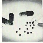
Microminiature pellet resistors are suited for use in flatpacks, microwave loads and attenuators, temperature compensated transistor circuits, etc. Pellets are available in three models measuring 0.100 x 0.062 in. Tolerances are attainable to  $\pm$ 1%, resistance range is 10 ohms to 500 kilohoms. Pyrofilm Corp., 60 S. Jefferson Road, Whippany, N.J. 07981 [248]
