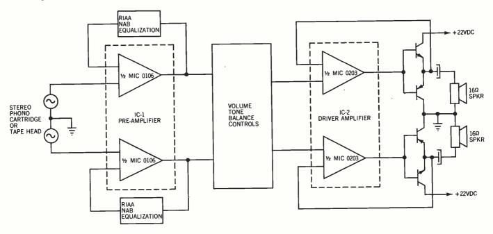
5 WATT STEREO AMPLIFIER UTILIZING MALLORY INTEGRATED CIRCUITS
