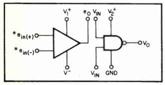
2. Improve your computer's memory with Linear Circuit 511. This one's a versatile transistor array. It's also a pre-amp – with DC characteristics that are 50 to 100% better than competing devices! Other memorable points: 1) low offset voltage  $\pm 2mV$ ; 2) low offset current; 3) single power supply; 4) AGC capability.
