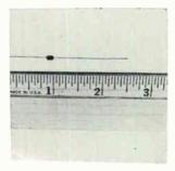
Microminiature, magnetically shielded axial lead inductor series designated the Pee-Wee Ductor is designed to meet MIL-C-15305C Class 5 requirements. It has minimum Q values of 34 to 55 at r-f frequency, with a standard inductance tolerance of  $\pm 10\%$ . Current capabilities range from 43 ma to 1% amps. Nytronics Inc., 550 Springfield Ave., Berkeley Heights, N.J. 07922 [344]
