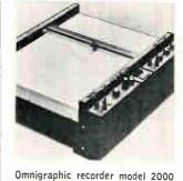
offers a convertible chassis and plug-in expandability. It will accommodate an X-Y, strip chart, T-Y or a variety of special designs in one main frame. Each X-Y can use 81/2 x 11 in. charts or 11 x 17 in. charts interchangeably. Sensitivity is 1 mv/ in., accuracy =0.2%. Houston Instrument Div. of Bausch & Lomb, Bellaire, Texas [363]
