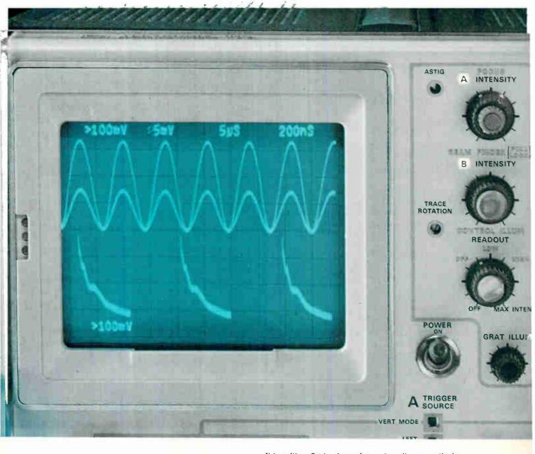
larly difficult with "fixed" readout devices). The display isn't limited to alphanumerics; such things as arrows, limit markers, and pictorial symbols can be included. And external information, not from the plug-in, can be mixed into the display.
