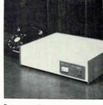
Data set TMX-202G interfaces with teletypewriter and business machines. It is a desk-top, singlechannel-end data set operating at rates to 1,800 bps. Digital interface meets RS-232, CCITT V24 or MIL-STD-188B specifications. Mean-time-between-failure is calculated at approximately 20,000 hrs. Collins Radio Co., 19700 Jamboree Blvd., Newport Beach, Calif. 92663 [424]
