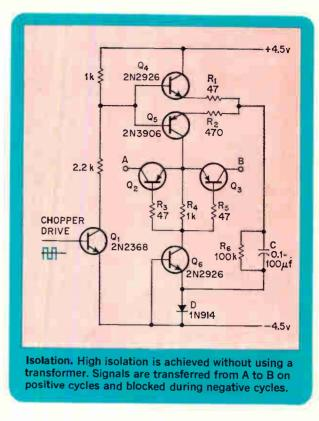
rest of the driving circuitry because  $Q_4$  and the diode are cut off.
