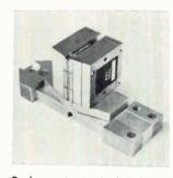
Dual-gap, nine-track, digital magnetic tape heads series HDG9 can be utilized for high density recording at 250 inches per second with fully compatible IBM formats. The series is composed of four models with packing densities of 3,200 flux reversals per inch at recording tape speed of 250 inches per second. Magnetic Head Corp., 95 Marcus Blvd., Hauppauge, N.Y. 11787 [427]
