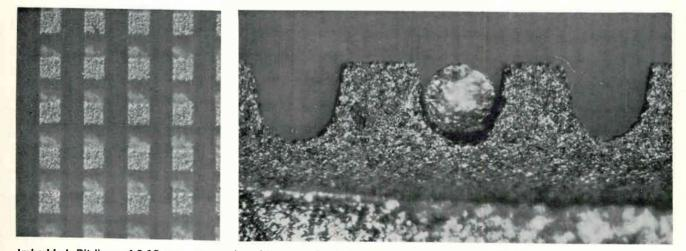
Imbedded. Bit lines of 0.13-mm copper wire with magnetic plating rest in shallow grooves. At right angles run 0.07-mm insulated copper wires, nestled in grooves cut deeper in ferrite keeper sheet.
