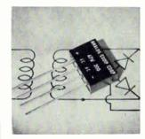
Full wave bridge rectifiers series AFW are pre-packaged silicon rectifier circuits for commercial and industrial applications. They directly replace individual units in multirectifier circuits. Units come in the following prv ranges: 50, 100, 200, 300, 400, 500, 600, 800, 1,000 v all with d-c output of 2 amps at  $50^{\circ}$ C ambient. Analog Equipment Corp., 18 Granite St., Haverhill, Mass. [439]
