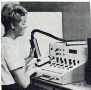
Thermospot probe model TP-200 measures h-f operational amplifiers over entire operating temperature ranges within minutes. It takes 15 to 60 sec to bring the component temperature from ambient to -55°C to up to ±125°C, depending on the device package. A dual-in-line ceramic package can be tested at -50° and +125°C in 90 sec. EG&G Inc., Goleta, Calif. [365]
