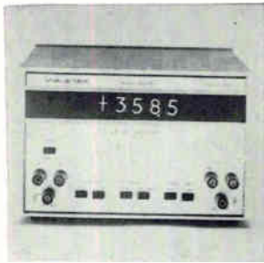
Precision digital phase meter model 750 features stable, long-term phase measurements. Frequency is 10 Hz to 1 MHz. Impedance is 1 megohm shunted by 30 pF. Recorder output is 0 to +3.6 V for 0° to 360°. Input voltage is 1 mV to 300 V rms. Resolution is 0.1°. Accuracy is ±0.1% full scale. Price is $1,500. Wavetek, P.O. Box 651, San Diego, Calif. [362]
