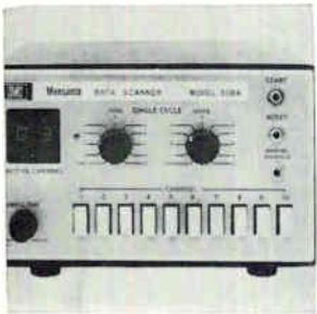
Four-pole, 10-channel reed switch matrix-data scanner 508A is suited equally to low-level guarded multiplexing of 3 or 4 analog signals and to 4-line-per-digit data transfer, commutation or steering. Its reed relays may be energized to connect a set of 4 input terminals to a corresponding set of 4 output terminals. Monsanto Electronic Instruments, W. Caldwell, N.J. [361]
