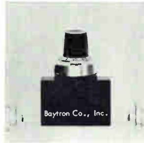
Dial calibrated variable phase shifter features a precision ball bearing mechanism with a differential drive counter that assures accuracy and reliability with fine readout definition. Model 3E-13 (60-90 Ghz) features calibration accuracy to \pm 3^\circ at any desired frequency. Vswr is rated at 1.20 max, with minimum phase shift of 180^\circ . Baytron Co., Medford, Mass. [403]
