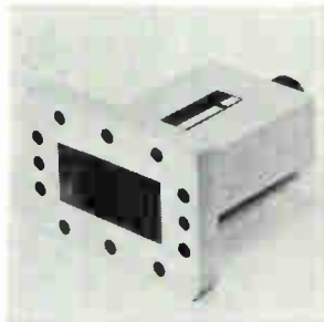
Waveguide-to-coaxial adapters WR229 feature an end launch configuration and provide extremely low vswr of 1.10 max. over the communication satellite band of 3.7 to 4.2 Ghz. They can be obtained with either precision N connectors (male or female) or the new high precision APC 7, 7 mm connector. Maury Microwave Corp., 8610 Helms Ave., Cucamonga, Calif. 91730 [407]
