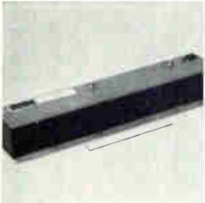
Microwave amplifier WJ-1115, covering 7 to 11 Ghz, is for use in airborne ecm or data link systems. It features integral power supply and provides 3 w power output, 45 db small signal gain and 22 db maximum noise figure in X-band. Unit weighs less than 6 lbs and comes in a package 2.3 x 3 x 16 in. Watkins-Johnson Co., Stanford Industrial Park, Palo Alto, Calif. [401]
