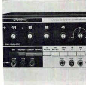
Precision calibrator model 311 offers 0.01% accuracy in both voltage and current. Five voltage and two current ranges are available and afford complete instrument calibration facilities. Current resolution is \mu a and voltage resolution is 1 \mu V. Rated load is 100 ma, which allows for use as a lab power source. United Systems Corp., 918 Woodley Rd., Dayton, Ohio 45403 [367]
