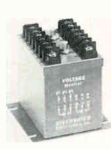
Three-phase voltage band monitors series PB protect electrical and electronic equipment required to operate between 2 voltage limits. Each of the 3 phases is monitored for an under or over voltage limit. The monitor can be used to sound an alarm, light warning lights, shut down or remove equipment from the line. Diversified Electronics Inc., Box 6231, Evansville, Ind. [383]
