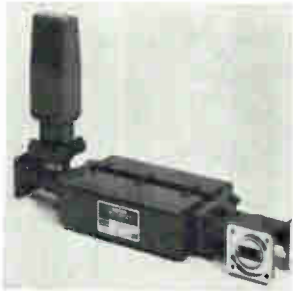
Four-part, differential-phase-shift circulator H62DA1 is for use as a duplexer or isolator in the frequency range of 15 to 17.5 Ghz. The unit can handle up to 1 kw of average power and up to 10 kw of peak power with a load vswr of 2:1. Cooling of the 4-lb circulator is through natural air convection. Varian Microwave Components Operation, 611 Hansen Way, Palo Alto, Calif. [406]
