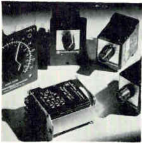
On/off temperature controllers series 9317 may be actuated by thermocouples or resistance temperature detectors. They contain solid state circuits in conjunction with a relay output. The output relay de-energizes when the setpoint temperature is reached and energizes after temperature falls below the setpoint. Sigma Instruments Inc., 170 Pearl St., Braintree, Mass. [381]
