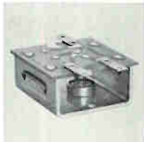
Series LAR line activated relays are for a-c power switching in single pole normally open uses. The series, utilizing a thyristor design, eliminates moving contacts, resulting in a highly reliable unit with virtually infinite switching life. Units are available in 4, 6, 8, 10, and 15-amp ratings for either 120 or 240 v a-c. Electronic Control Corp., P.O. Box J, Euless, Texas [342]
