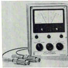
Electronic micrometer series 300 is capable of non-contact measurement of objects with a resolution of 0.000010 in. The objects being measured may be either stationary or moving. Meter readout as well as ±5 V analog output is available. Unit is designed to provide a continuous 100% inspection of production pieces. Lion Research Corp., 60 Bridge St., Newton, Mass. 02195 [363]
