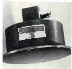
Cavity-backed Archimedes spiral antennas are broadband units that are circularly polarized with essentially constant impedance and radiation characteristics. Model S6510 illustrated operates over the 2 to 11 Ghz range. Nominal performance characteristics are: gain, 5 db; vswr, 2:1; axial ratio, 2 db; and beamwidth, 75^\circ . Eastern Microwave Corp., 139 Swanton St., Winchester, Mass. [408]
