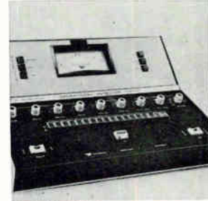
Operational amplifier tester model 5104 offers rapid testing of 15 op amp parameters in either a full automatic mode (200 msec/test) or by push-button selection from the front panel. Meter scaling, power supply voltages, and test conditions are available as front panel controls. Price is $4,500. Philbrick/Nexus Research, Allied Dr. at Route 128, Dedham, Mass. [368]
