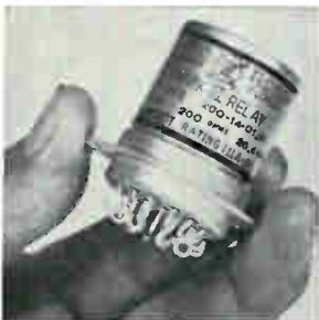
Six-pole double-throw relay series 200 Mark II can operate continuously at up to 200°C. It conforms to MIL-R-5757/11. Its contact mechanism delivers a positive wedge-wiping action that cuts through surface films to create a continual self-cleaning of the precious metal contacts during make and break movements. KDI Electro-Tec Corp., Ormond Beach, Fla. [345]
