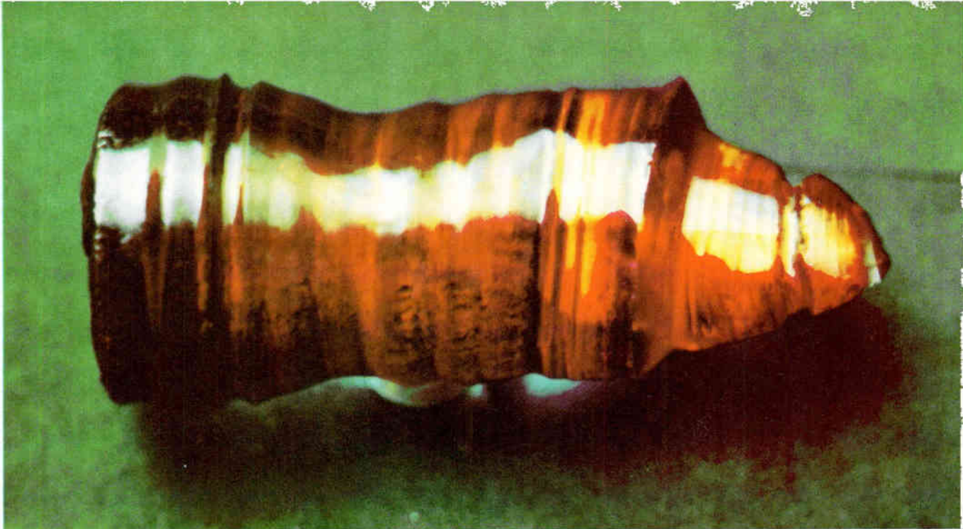
Growth plan. This crystal of bismuth germanium oxide was grown by the Czochralski pulling technique. Crystals 6 inches and longer are becoming available that will provide delays of 100 microseconds.
