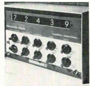
Electronic predetermining counter 7122 Econo-Flex with 5 counting decades features illuminated digital display, and the design assures continuous counting in the event of a display failure. The counters operate and automatically recycle at speeds to 10,000 counts/sec, accepting input from photoheads, contact closures, or direct pulses. Veeder-Root Co., Hartford, Conn. [384]
