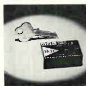
Video amplifier model VA-21 provides a slewing rate of 750 v/ \mu sec with a 12 Mhz frequency for full output. Its ultrastable 6 db/octave roll-off characteristic insures a useful gain-bandwidth product of 80 Mhz minimum. It offers an output of \pm 20 ma at \pm 10 v, 20 \mu v/ ^{\circ} C voltage drift and 0.5 na/ ^{\circ} C current drift. Data Device Corp., 100 Tec St., Hicksville, N. Y. 11801 [384]
