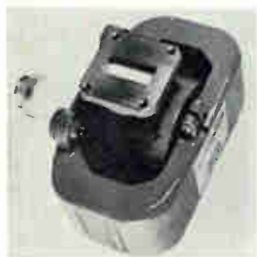
Coaxial magnetron SFD-377A delivers a peak output of at least 70 kw at a frequency between 9.355 and 9.395 Ghz. It is designed to meet difficult pulse applications. Pulse-duration capability ranges from 0.3 to 5.1 \mu sec, and the range of the rate of voltage rise extends from 90 to 160 kv per \mu sec. S-F-D Laboratories, 800 Rahway Ave., Union, N.J. 07083 [402]
