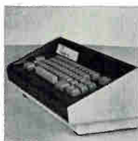
Solid state alphanumeric keyboard features a Neverwear non-contacting key switch. Coded capacitance keys provide improved reliability and an output compatible with TTL or DTL. The keyboard needs no anti-bounce circuitry, and any popular code may be used. The flexible, modular unit is priced at $100. Data Term Inc., 1611 Manning Blvd., Levittown, Pa. 19057 [423]
