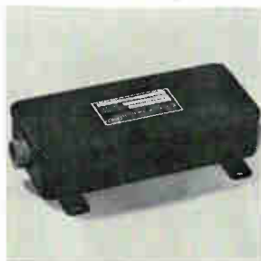
Voltage and frequency monitor 35-73-01840 operates within the band 380 hz to 420 hz \pm 5 hz. It senses voltage and frequency of the power source and, if they remain within proper values, holds an internal relay energized to provide a fail-safe operation. Frequency sense is 40 to 2,000 hz; voltage sense, 20 to 500 v. Electronic Resources Inc., 4561 Colorado Blvd., Los Angeles [406]
