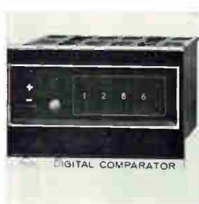
Panel-mounted digital comparator model 4310 provides on/off control by comparing BCD input data to a preselected limit. It will compare on command, with comparison to input data being transferred to the output when a compare command pulse is received, or can compare continuously. Price for adjustable limit models is $165. API Instruments Co., Chesterland, Ohio. 44026 [422]
