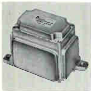
Vibra-Larm detectors series IVA-100 provide automatic warning or shutdown due to excessive vibration. They feature a built-in time delay, an on-off trigger output, and an adjustable alarm-set-level. Frequency response is from 5 to 1,000 hz with a temperature range from -40^{\circ} to +170^{\circ} F. Repeatability is within 1% of setting. Columbia Research Laboratories, Woodlyn, Pa. [381]
