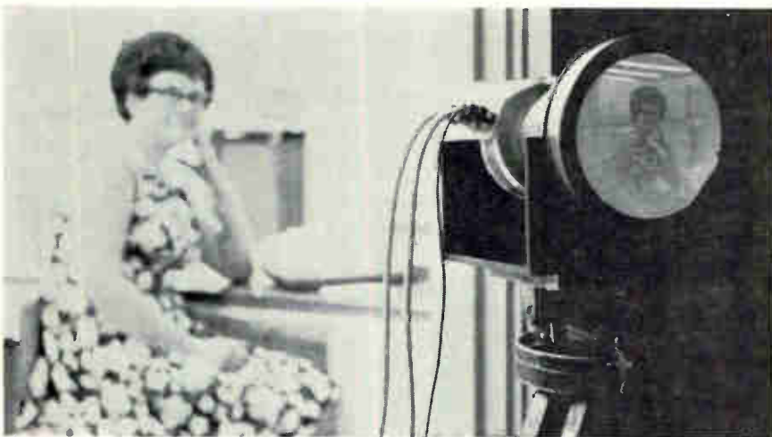
Picture this. Aerojet Delft's direct-vision display tube will enable soldier, sailor, or airman to use starlight scope without pressing his eye to it.
