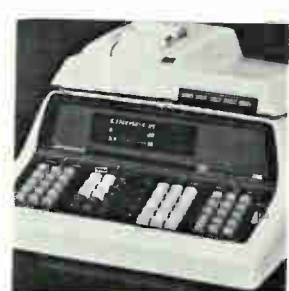
Calculator printer model 9120A prints at 180 lines per minute with about as much noise as the ticking of a clock. It has an assembly consisting of 7 tungsten print fingers which sweep across the width of the paper in a vertical array. Characters are written by sending short bursts of very low current through the proper stylus fingers. Hewlett-Packard Co., Palo Alto, Calif. [428]
