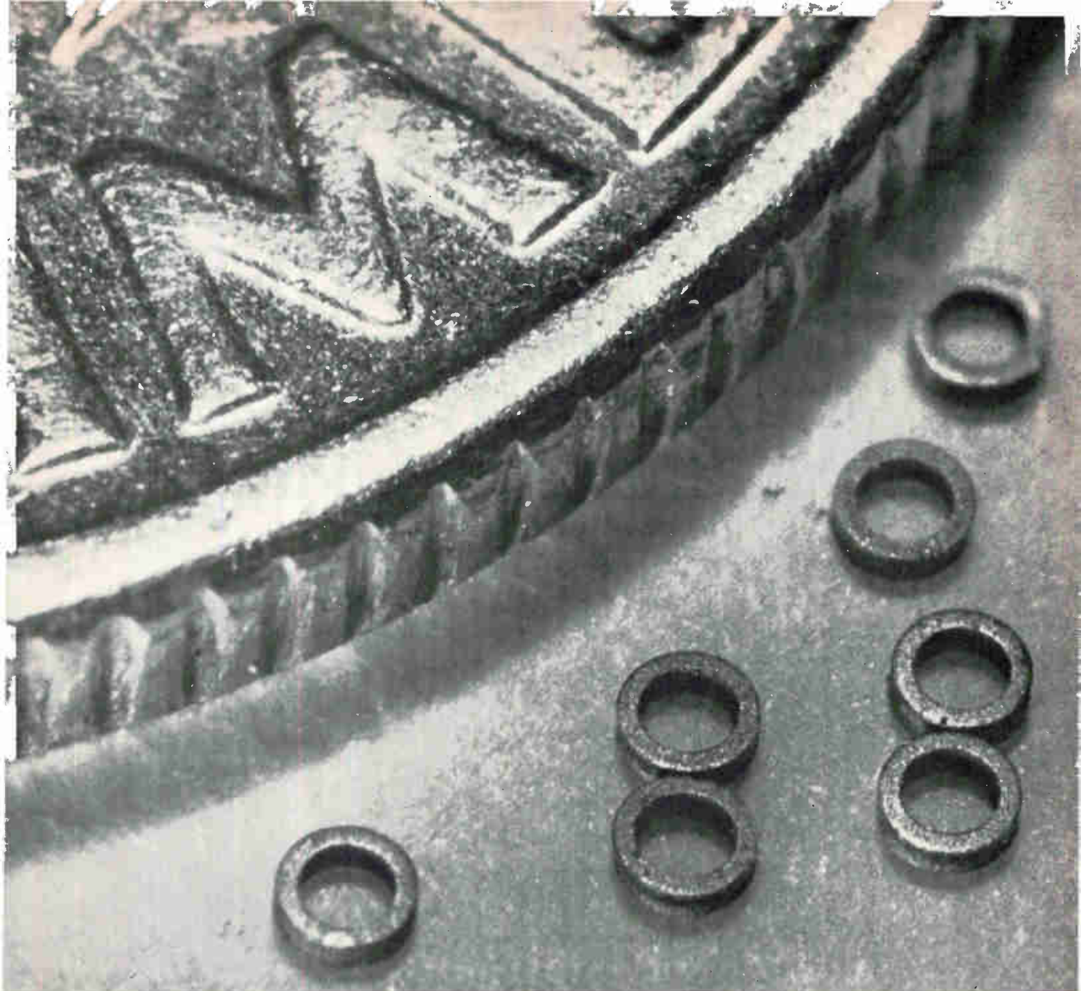
Unretouched photo of U.S. dime and Data Products' 18-mil cores.
