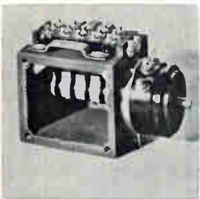
Potentiometer-microswitch module features 7 amp, 250 v snap-action microswitches, phased to the 7/8 -in. diameter precision potentiometer contact at arbitrarily prescribed angles. The potentiometer features rugged construction and provides linearities as close as 0.25% with a resistance range of 500 ohms to 150 kilohms. New England Instrument Co., Natick, Mass. [385]
