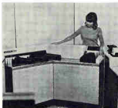
Data gatherer. Optical character reader takes information from small cards for input to computer.
