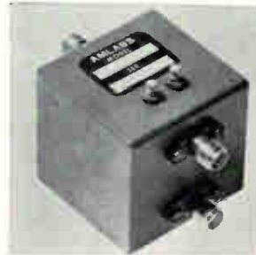
Dual 2-stage YIG filter model C2202 is for use at C-band frequencies. It operates from 4 to 8 Ghz. Guaranteed r-f performance, per 2-stage channel, includes 2.5 db insertion loss, 3 db-bandwidth points within 30 to 50 Mhz, and off-resonance isolation greater than 60 db. Unit measures 1.2 cu in. Advanced Microwave Labs, 611 Vaqueros Ave., Sunnyvale, Calif. 94086 [403]
