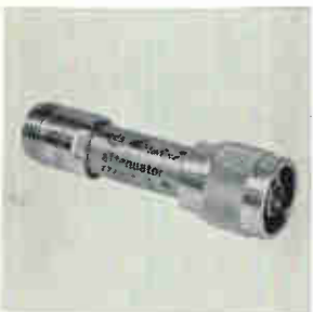
Fixed coaxial attenuators have values of 3, 6, 10, and 20 db. The 3- and 6-db values are flat to within \pm 0.2 db throughout the frequency range from d-c to 12.4 Ghz. The 10- and 20-db values hold to within \pm 0.2 db from d-c to 6 Ghz, and to within \pm 0.3 db from 6 to 12.4 Ghz. Vswr is 1.15 from d-c to 6 Ghz, 1.20 above that. Narda Microwave Corp., Plainville, N.Y. [405]
