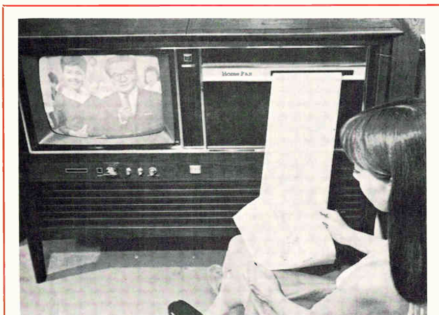
Stay at home. Japan's Matsushita, to drum up interest in consumer facsimile, has developed three systems for home reception. One (above) puts signals in the tv vertical retrace period to generate two pages a minute. The second builds up a fax line from short signals at the end of horizontal lines. The third uses empty space in f-m signals.
