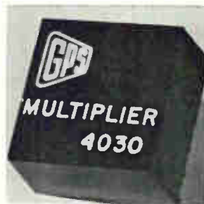
Hybrid linear circuit multiplier model M-4030 measures 1.12 \times 1.12 \times 0.4 in. It has a total accuracy of 1%, including errors due to linearity, scale factor and offset. Bandwidth is 1.5 Mhz with a slewing rate of 15 v per \mu sec. Feedthrough is less than 30 mv peak-to-peak at 50 khz. Output noise is below 1 mv rms. GPS Instrument Co., 14 Burr St., Framingham, Mass. 01701 [383]
