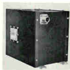
Four-stage, current-tuned YIG filter operates over the 12.4 to 18 Ghz spectrum. Features include a 3 db nominal bandwidth of 275 Mhz, 4 db insertion loss, 1.5:1 vswr, and rejection of 24 db per octave. Additional parameters include cold isolation 60 db, passband ripple (including spurious) 1 db maximum. Frequency Engineering Laboratories, Farmingdale, N.J. 07727 [407]
