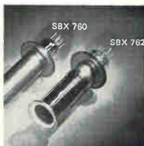
Vacuum ultraviolet photomultiplier tubes SBX-860 and SBX-762 are calibrated as secondary standard detectors in the 2,000 to 1,150 angstrom wavelength range. Both have extremely uniform and stable characteristics when operated in the pulse-counting mode, which permit them to be used for fluxes from 1 to 10^9 photons/sec/cm 2 . Bendix Research Labs, Southfield, Mich. [342]
