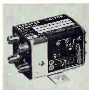
Coaxial transfer switch series 09-51 has a vswr at 12.4 Ghz of 1.25:1, and provides high interchannel isolation from 0 to 18 Ghz. Remote actuation is of the latching type, requiring no holding current. Actuating current is 53 ma at 26.5 v at 25°C. for latching and 177 ma for fail safe operation. Electronic Resources Inc., 4561 Colorado Blvd., Los Angeles 90039 [347]
