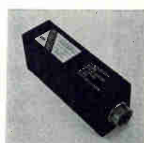
Power converter PS-274 is designed to provide 5-v d-c power for aircraft instrument lighting systems. Operating from the 28-v aircraft power source, this unit provides an output that may be remotely adjusted from 0 to 5 v. The output current capacity of 7.5 amps nominal provides power for 125 60-ma lamps or 65 115-ma lamps. EMP Electronics Inc., Box 2346, Phoenix. [388]
