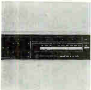
Coincident-current core memory system VersaStore IV operates asynchronously with a full cycle time of 900 nsec and an access time of 350 nsec. One model has a storage capacity of 4,096 words of 40 bits, or 8,192 words of 20 bits, and a larger model can store up to 8,192 words of 40 bits or 16,284 words of 20 bits. Varian Data Machines, 2722 Michelon Dr., Irvine, Calif. [426]
