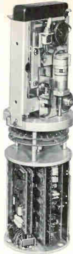
Oceanographic applications module with tape recorder, analog-to-digital converter, output register, programmer and multiplexer.
