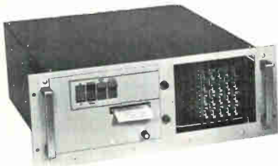
Printed circuit boards, with easily accessible switches permit unusual flexibility for Programmable Zero Suppress.
