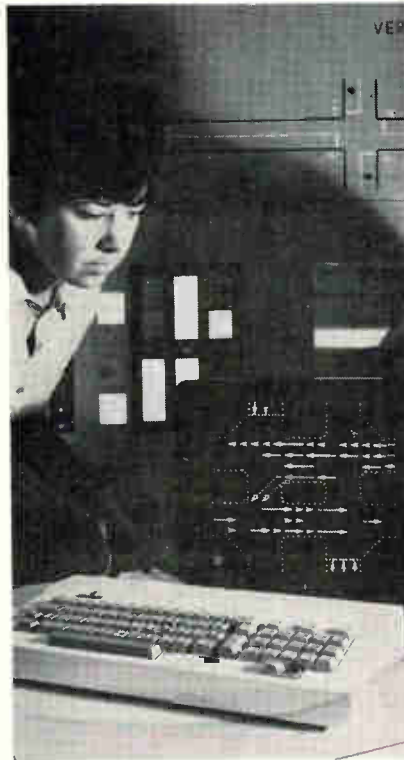
Under control. Traffic flow is analyzed and directed by Siemens computer. Display helps in simulation.
