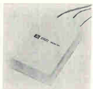
Direct connected modem DCM-151 provides serial data transmission up to a 150 baud rate. It connects directly to private or leased voice grade telephone lines up to a distance of 5 miles. The data input/output levels comply with EIA RS-232B, and the fsk tones are transformer coupled to the transmission lines. Anderson Jacobson Inc., 2235 Mora Dr., Mtn. View, Calif. [428]
