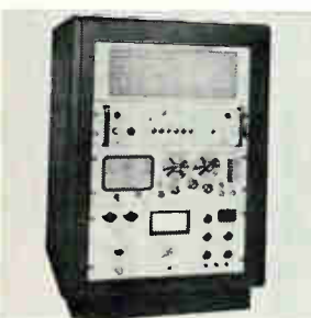
Sweeper/signal generator model M402S provides an all-electronically-swept output of up to 100 watts at any frequency, or over any band of frequencies, from 200 khz to 220 Mhz. Unit is designed for laser research, rfi testing, nuclear magnetic resonance work, and electronic countermeasures. Instruments For Industry Inc., 151 Toledo St., Farmingdale, N.Y. [365]
