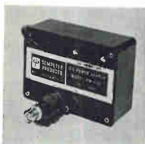
Bench model power supply PM429 has a case size of 1.63 x 2.88 x 4 in. Its binding posts are spaced to accept a standard BNC to banana plug adapter. Output is 5 v d-c at 250 ma. Line and load regulation is \pm 0.05\% each and ripple and noise is 0.5 mv rms. Price (1-9) is $45.60, (100-299) $34.40. Computer Products Inc., 2709 N. Dixie Highway, Fort Lauderdale, Fla. [386]
