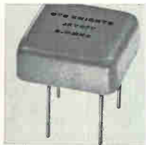
Crystal oscillator model JKT0-77 for p-c board applications is suited for computer clocks and other timing devices. A frequency range of 5 Mhz to 20 Mhz is available. Measuring 1 x 1 x 3/8 in., the unit withstands shock and vibration per MIL-STD-202. Input supply requirement is +5 v d-c \pm 5\% at 20 ma max. CTS Knights Inc., Sandwich, Ill. 60548 [345]
