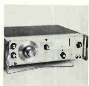
Generator model F323A is a 10 hz to 10 Mhz unit that serves not only as a low distortion sine wave oscillator but also as a sine and square wave function generator. Square wave output is provided simultaneously and has a rise time of less than 10 nsec. Extremely flat frequency response is also featured. Price is $660. Data Royal Corp., 8014 Armour St., San Diego, Calif. [368]
