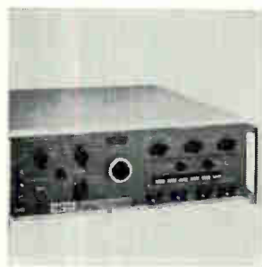
Servo system analyzer model 199 is for analysis and test of servo-mechanisms and complex control systems by observing phase and amplitude response with respect to various frequencies and wave shapes. Harmonic distortion is less than 0.5%. Phase accuracy is ±1° from 0 to 360°. Frequency accuracy is ±1%. Servo Corp. of America, 111 New South Rd., Hicksville, N.Y. [362]
