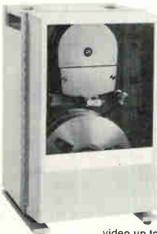
PI-7100 Video/Instrumentation Captures video, radar, RF, multiplex, telemetry . . . any broadband data up to 1.5 MHz, or video up to 3.5 MHz. Operates for 90 minutes on a 10½" reel of tape using helical scan transport. Includes VariScan™ and StopScan™ playback.
