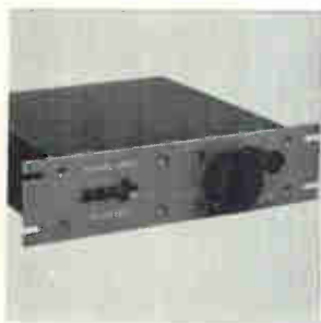
Digital precision angle transmitter model 2500T is used to transmit and indicate an angular position of a potentiometer, synchro or resolver. It has 360° for angular position with 0.2° resolution. The digital indicators which prevent parallax can be read in tenths of a degree or in minutes or seconds (as specified). Occo Mfg. Corp., 8 Romanelli Ave., South Hackensack, N.J. [381]
