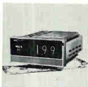
Digital panel meter model 1260 is available in voltage ranges of from 0-199 mv to 0-1 kv and in current ranges of from 0-19.9 µa to 0-199 ma. Features include ±0.5% full scale ±1 digit accuracy, 25% over-range, and a circularly polarizing window filter. Price is under $100 in quantities of 25. Weston Instruments Inc., 614 Frelinghuysen Ave., Newark, N.J. 07114 [366]
