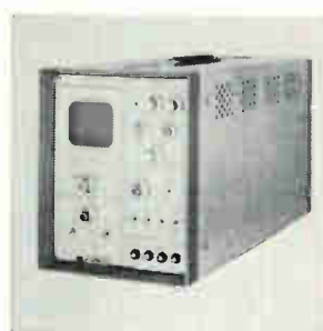
An industrial version, called model 900, of the CAT (computer of average transients) is capable of separating data in 1,024 channels into signals and eliminating background noise. Repetition rates are from about 60 per sec to once in 31 msec. Memory capability is 999,999 in each channel. Price is $6,490. Technical Instruments Inc., 441 Washington Ave., North Haven, Conn. [363]
