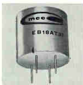
Audio output transformers provide isolation and impedance matching for popular power integrated circuits in 1/2 to 1 watt power output range. A choice of single-ended or push-pull input is offered. The epoxy encapsulated units are for plug-in on standard 0.1-inch grid spacing. Magnetic Circuit Elements Inc., Del Monte Research Park, Monterey, Calif. [343]
