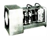
Crt mount is precisely fabricated to accomplish the accurate alignment required in high resolution work with 10 in. flat face crt's. For maximum rigidity, the mount is constructed of heavy-duty cast aluminum. Complete magnetic shielding of crt and magnetic components is achieved by a 3layer shield assembly. Syntronic Instruments Inc., Inlustrial Road, Addison, III. [346]
