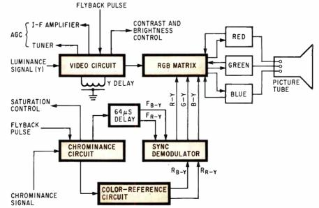
**Colorful quintet.** Color-tv signals from video i-f amplifier are processed by five IC's and two delay lines. Sync demodulator and matrix are in mass production. The other three should be in production next year.
