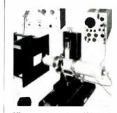
Microspot crt analyzer MA100 is rugged, and suitable for either laboratory or production quality control use. Resolution measuring methods include spatial frequency, two slit, light intensity distribution, and half power line width. A change in the graticule is all that is needed to shift from one method to another. Ferranti Electric Inc., E. Bethpage Rd., Plainview, N.Y. L3681
