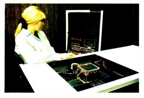
Test station. Core memory on the fixture in the foreground is checked, and error location pinpointed by numerical readout and cathoderay-tube display. The station can also include printer output of type of error and its location.
