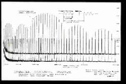
Typical 7899 System X-Y Plot of conducted interference from 250 kHz sinewave pulsed at a 10 kHz for a duration of 12m sec.
