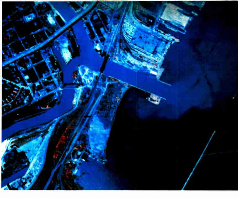
Laser-beam picture. Aerial view of Cleveland waterfront was made from a 35 mm color-infrared transparency by RCA's 2-inch return-beam vidicon/laser reproducer system. The vidicon took a separate picture of the transparency through three color filters. Over-all system resolution is 4,500 tv lines and video bandwidth is 4 Mhz. Scan-like lines, caused by jerky movement of film under laser, will be eliminated.
