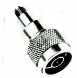
Attenuating adapter model AH-EO1 is essentially an adapter from type N to 3 mm with a built-in 10 db attenuator. It reduces hardware in a circuit by combining two elements, thus eliminating a source of error or instability. Unit operates from d-c to 4 Ghz and is available in attenuation values to 20 db. Price is \$50. Microlab/ FXR, Ten Microlab Road, Livingston, N.J. [405]
