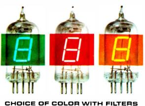
Simple filtering provides an almost unlimited choice of colors for identifying individual readout arrays.
