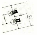
Plastic transistors for 20 and 35 w complementary audio amplifiers measure 5/8 x 1/2 x 1/8 in. The npn MJE205 and pnp MJE105 are 5 amp units with a  $V_{\text{CEO}}$  of 50 v, power dissipation of 65 w. The npn MJE2801 and pnp MJE2901 are 10 amp units with a  $V_{CEO}$  of 60 v, P<sub>D</sub> of 90 w. Prices range from \$1.25 to \$1.95. Motorola Semiconductor Products Inc., Box 20924, Phoenix 85036. [440]
