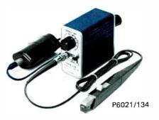
The P6021 AC Current Probe and Type 134 Amplifier provide the facility for accurate current measurements over the wide range of 12 Hz to 40 MHz without breaking the circuit under test. Used with any plug-in unit having a deflection factor of 50 mV/div, the P6021/134 provides deflection factors from 1 mA/div to 1 A/div.
