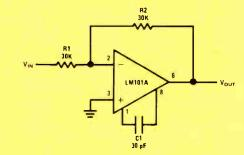
FIGURE 1. Standard Frequency Compensation
