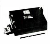
Solid state TR switch S255 is used with a fixed circulator in pulsed radars to alternately connect the transmitter and the receiver to the antenna. Switching time is less than 0.5 #sec; switching energy required, 30 microjoules. Unit handles 10 kw peak continuously and up to 100 kw for short durations. RCA/Electronic Components, 1000 S. Seconc St., Harrison, N.J. 07029. [403]
