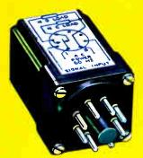
■ Universal AC or DC control voltage with complete circuit isolation from load switching circuit. ■ Externally-adjustable pull-in voltage level from 80-130V AC or DC, with close differential between pull-in and drop-out where accurate voltage sensing is required. ■ Control of high inrush lamp, inductive or normal resistive loads from 10 ma to 3 amps. ■ Internal filtering prevents random turn-on of "off" contacts.
