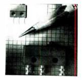
Precision, snap-action switches measure only 0.3 x 0.2 x 0.1 in. exclusive of terminals. They are rated at 1 amp resistive at 28 v d-c or 115/250v a-c, with an electrical life of 100,000 cycles and a mechanical life of 500,000 cycles minimum. Operating temperature range is from  $-100^{\circ}$  to  $+250^{\circ}$  F. Hi-Tek Corp., 2220 S. Anne St., Santa Ana, Calif. 92704. [343]
