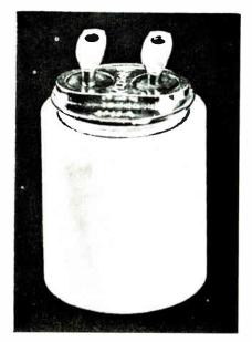
Safeguard. Switch is mounted in a container made of beryllia—a heat-conductive electrical insulator.
