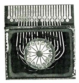
Two keys. The ferroelectric wafer, when embedded in opaque epoxy, makes a key that's much harder to duplicate than the old-fashioned variety.
