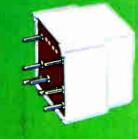
■ Unique, compact design. ■ All terminals on .1 grid spacing for standard printed circuit board. ■ Solders right on PC board. ■ Conforms to UL requirements for Business Machines. ■ I watt normal power—½ watt on request. ■ 3500 OHMS coil resistance (120V AC-60Hz). ■ Standard voltages 6 to 120 AC—6 to 24 DC. ■ Mechanical life over 10,000,000 operations. ■ 3 AMP. resistive 115V. 60Hz contact rating.
