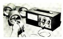
Finding flux. The 505, a portable instrument, can be used to check out the permanent magnets in motors.
