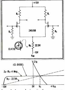
In a balanced circuit the commonmode gain is decreased in approximate proportion to the ratio of source resistances. By substituting the Siliconix CL4710 for the 22.5K source resistance,  $R_s$  is raised to 4 megohms. Common-mode gain is decreased by a factor of over 100. For further information and immediate applications assistance, call the number below. Ask for exten-
