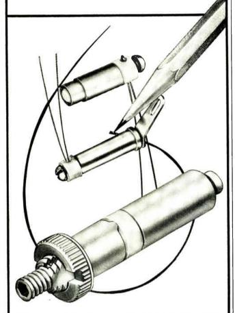
These new trimming capacitors are ideally suited for VHF and UHF applications requiring low minimum capacity and delta C. They provide high resolution and are electrically stable. Tuning is linear. High Q (2000 at 1 mHz typical). Insulation resistance 106 megohms. Temperature range--55° to +150°C. Voltage breakdown 2000 VDC. Part numbers 273-1-1 and 273-1-2 nominal capacity .25 pf min., 1.5 pf max.; part 273-15-1 nominal .30 pf min., 2.9 pf max.
