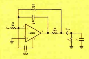
FIGURE 7. Capacitive Load Isolation
