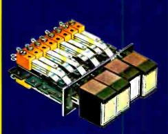
■ Sleek, compact design—only 1<sup>1</sup>/<sub>8</sub>" high. ■ Non-illuminated or illuminated with color coding. ■ Buttons on %" centers. ■ Up to 12 stations in multiples of 2. ■ Contacts rated at both 1<sup>1</sup>/<sub>2</sub> amp and 10 amps at 115V AC resistive. ■ Up to 4 pole double throw per station. ■ .110 Quick Connect Terminals. ■ End panel has four %<sub>32</sub>" tapped mounting holes. ■ Long life—100,000 mechanical operations.
