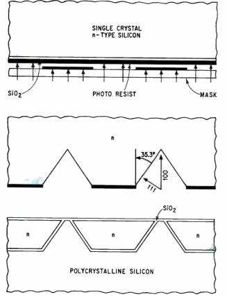
Isolation steps. Pattern is exposed to back side of silicon slice during dielectric isolation. Then unexposed regions are etched with anisotropic etchant, which forms v-shaped groove. SiO<sub>2</sub> dielectric coats single crystal; polycrystalline silicon backfills grooves, and silicon is lapped from top to expose grooves.
