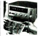
Digital counter PM-6630 is a 160-Mhz unit that measures pulse width and delay, as well as frequency to 10 nsec resolution. It allows users to select digit and stability options that tailor the unit's performance to their specific application or budget. Price of the 8-digit version is \$2,795; the 6-digit costs \$2,20. Philips Electronic Instruments, S. Fulton Ave., Mt. Vernon, N.Y. [363]
