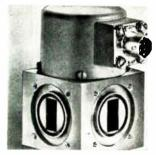
Ku-band, 3-port waveguide switch model NMC-5071 offers greater than 90 db isolation and measures only 2.75 in. in height. The unit has a low insertion loss of 0.2 db, and a low vswr of 1.10. It is available in 2-, 3-, and 4-port design. The switch measures  $1.750 \times 1.750 \times 2.75$  in. and weighs 14 oz maixmum. Neico Microwave Co., 211 Second Ave., Waltham, Mass. 02154. **[404]**
