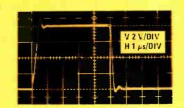
FIGURE 5. Large Signal Transient Response with Feedforward Compensation
