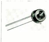
Silicon photodiodes come in 2 types. Type 720, for industrial control use, offers a minimum light current of 90 µa at 500 footcandles 2800°K, maximum reverse dark current of 1µa at -1 v. The 820 is for low noise and faster response uses. Both have a peak spectral response at 8,500 A. Price ranges from 69 cents to \$2. National Semiconductors Ltd., Plattsburgh, N.Y. [438]
