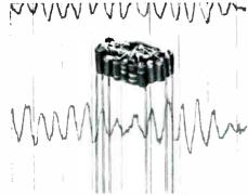
Enlarged approximately 1½ times When you convince more than 30 discrete components, including 10 electrolytic capacitors ranging from 0.01 to 2.2 mfd., to huddle together in a space somewhat smaller than 1/20 of a cubic inch, you've got yourself some pretty high-density packaging.
