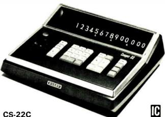
Fourteen digit, 6 decimal place capacity. Automatic decimal and half-cent round off system. Credit balance. Two working registers plus a memory bank. Automatic constant multiplication and division. Memory indicator, over capacity error light. Silent, versatile and very elegant. Just 8.8 lbs.
