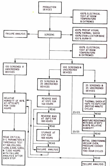
**Proposition.** The test program proposed to makers of plastic-encapsulated IC's by the Rome Air Development Center is designed to produce data on failure modes for such devices. Assemblies will be put through four screens before they're run through the program, which is sequential. The way the checks are set up, a total of 100 screened and unscreened parts, stressed three ways, are subjected to a final 7,500-hour series of tests.
