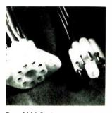
Type 1664-9 plug, used with the 1412 socket, makes a dependable circular connector. Male terminals snap-lock into their nylon housing but can be easily removed with a simple tool. The socket housing can be screw mounted or can be provided with integrally-molded mounting ears for fast snap-in chassis assembly. Molex Products Co., Downers Grove, III. [341]
