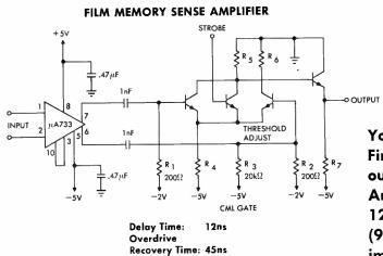
You might not have to build it after all. First check out the Fairchild  $\mu$ A733, our latest wideband Differential Video Amplifier. The 3dB bandwidth is 120MHz at a closed-loop gain of 10 (90MHz at a gain of 100). Input impedance is 25k $\Omega$ , phase linearity
