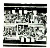
Hex 1-input inverters have been added to the SUHL I and II IC lines. The SG370 circuits operate at 12 nsec typical propagation delay and 22 mw power dissipation per gate function. The SG380's are rated at 6 nsec delay and 22 mw power dissipation. Units come in 14-lead hermetic flatpack or dual-in line ceramic packages. Sylvania Electric Products Inc., Woburn, Mass. [436]
