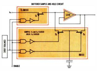
Low input leakage of the L120 OP AMP makes it ideally suited for sample-and-hold circuits. Two channels of this circuit require only three DG133s and one L120. An alternative approach would require two DG129s and one L120 for two channels.
