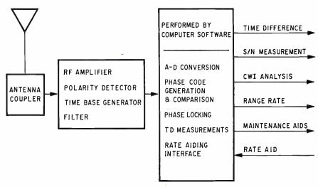
Simplicity itself. Litcom's 6-pound loran receiver has minimal hardware since most conventional operations are handled by airborne computer.
