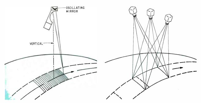
**Ground sweep.** The return beam vidicons would focus on the same part of the ground track beneath this spacecraft, but Hughes' multispectral camera would scan across the track with an oscillating mirror.
