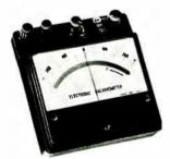
Portable electronic galvanometer type E11.501 incorporates stable solid state circuitry in a highly sensitive (10  $\mu$ v/div.) device with a 3 second response time. Unit features a common mode rejection of greater than 140 db at d-c, 50/60 hz, and an input resistance of approximately 9 kilohms. Price is \$135. Voltron Products Inc., 403 S. Raymond Ave., Pasadena, Calif. 91101. [365]
