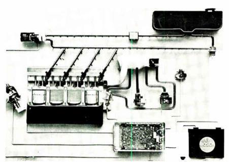
Around the loop. Fuel injection system, with control circuitry from Bosch, improves engine performance, lowers gas consumption, and reduces emission of exhaust contaminants to levels lower than are possible with carburetors.
