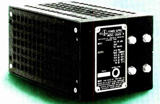
Optional 10<sub>µ</sub> sec. overvoltage protection. ■ Requires no external heat sink in ambients to 71° C. ■ 29 models—voltages to 330 Vdc at power levels to 300 watts. ■ Remote programming—remote sensing—series/parallel operation. ■ Overload and short circuit protection. ■ Meets military specifications.
