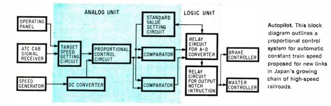
data on the presence of a train stored in the memory will not be erased even if the detection unit aboard the train fails. If the memory indication were erased, the proceed signal sent to the following train would probably result in a tailend erash.
