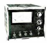
Log amplifier model 6001 accepts any r-f input from 400 khz to 130 Mhz with a power range of -70 dbm to +20 dbm. It provides a linear detected output for oscilloscope, voltmeter, or graphic recorder presentation. The output is accurate to  $\pm 3$  db. Packaged in a half-rack cabinet, the unit measures 8<sup>1</sup>/<sub>2</sub> 7 x 12<sup>1</sup>/<sub>4</sub> in. Telonic Instruments, 60 N. First Ave., Beech Grove, Ind. [364]
