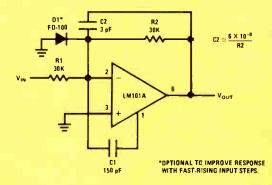
FIGURE 2. Feedforward Frequency Compensation
