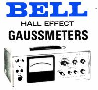
Model 640 A high performance incremental gaussmeter with precalibrated and interchangeable probes. Center zero meter for direct readout for small incremental variations in both  $\pm$  direction. 1.0% accuracy to 30 kG (0.5% to 10 kG). One volt FS calibrated output.
