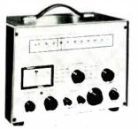
Precision bridge model 2785 is for measuring capacitance, inductance, resistance and Q. A built-in generator provides all the voltages needed. The instrument is accurate to within  $\pm 1\%$  on most resistance and capacitance ranges and to within  $\pm 1.5\%$  on most inductance ranges. Q measurements have a maximum error of  $\pm 5\%$ . Simpson Electric Co., 5200 W. Kinzie St., Chicago 60644. [366]
