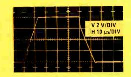
FIGURE 6. Large Signal Transient Response with Standard Compensation
