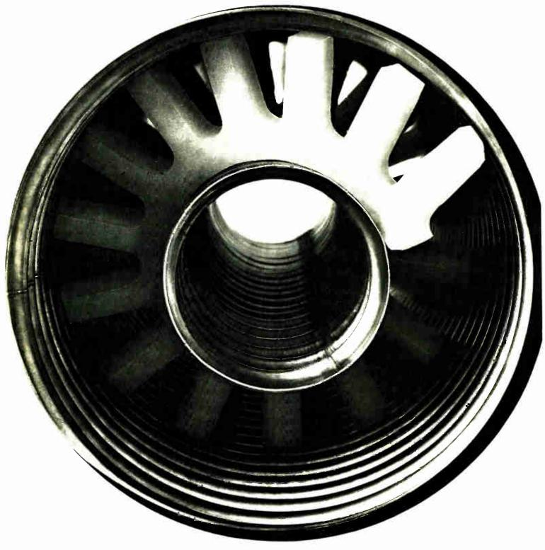
Faced with carrying a couple of hundred RF kilowatts? Need low, low attenuation? Move up to 8" HELIAX<sup>®</sup> coaxial cable. Big. Semi-flexible. Continuous lengths to 850 feet. Eliminates connector bullets and complicated hangers. Thermal expansion and contraction don't faze it. Power capabilities: 300 kw average at 30 MHz; 58 kw at 600 MHz. Use for HF; Tropo; OTH radar; VHF and UHF-TV. Wouldn't you like to know more? Communicate with Andrew.
