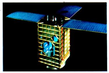
With windows, RCA's earth resources satellite would be a somewhat larger version of the company's Tiros M weather satellite. The ports in the craft are for the sensors including three 2-inch return beam vidicons.
