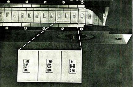
Hole filler. Chain module with magnetic character font for Potter printer. System replaces punched cards with man-readable letters.
