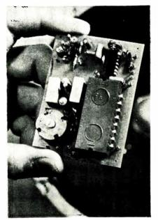
**Cool.** Mullard's experimental pdm circuit (black dual in-line package at top) and the power pack paired with it switch so efficiently that this 30-watt audio amplifier needs no heat sink. stand a 30-watt hi-fi amplifier based on an experimental pdm integrated circuit.
