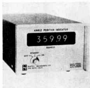
Dual-speed, automatic-ranging angle position indicator model 4062A can handle 1:36 and 1:10 two-speed synchro inputs. It offers several automatic features including 60 and 400 hz operation, 26 v and 115 v reference (rotor) amplitudes, and 11.8, 90, or 115 v rms line to line stator voltages, all available in one package. Natel Engineering Co., 7129 Gerald Ave., Van Nuys, Calif. [366]
