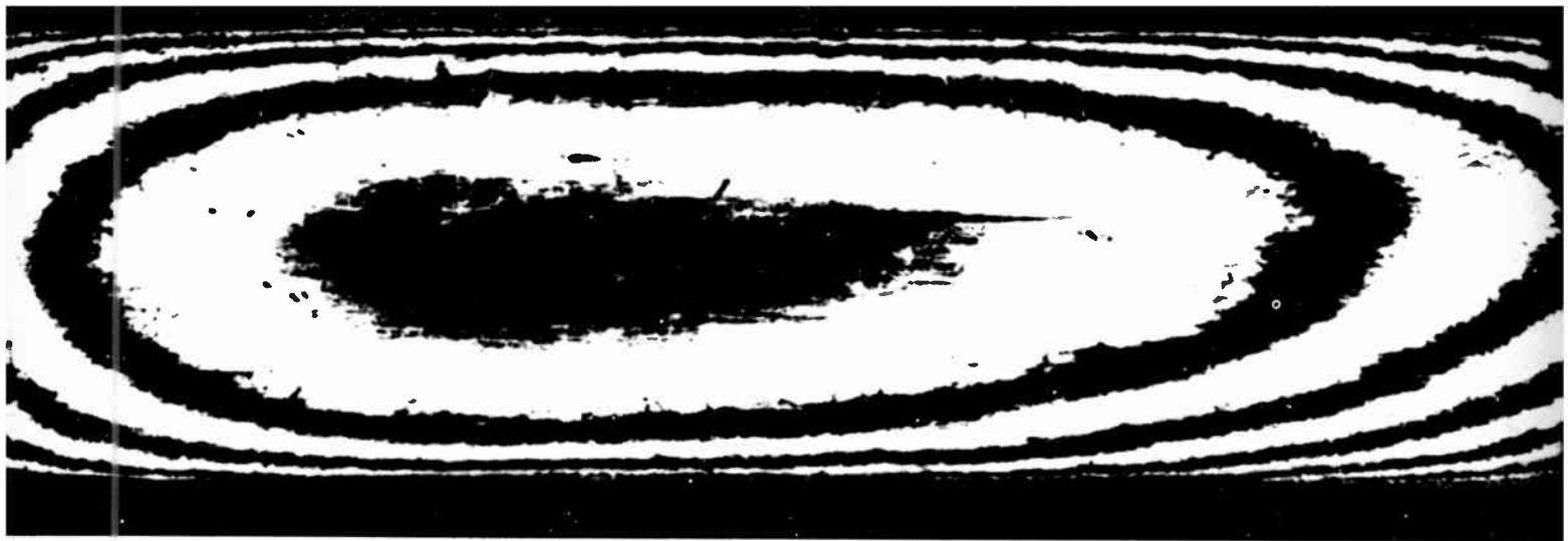
Interference photomicrograph of a gage block surface. Fringes give a clear picture of a surface drooping toward the edges.
