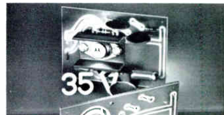
The new MC1561/1461 voltage regulators can handle inputs of up to 35-volts.
