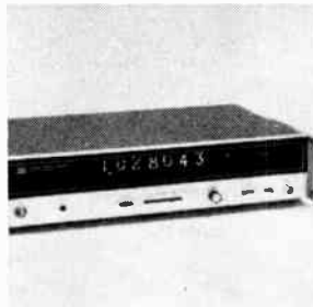
Automatic counter model 5323A has a range of 0.125 hz to 20 Mhz. It can measure the carrier frequencies of pulsed r-f or tone bursts, even those that are but a few microseconds in duration, without the use of a transfer oscillator. The unit is priced at $2,150. Deliveries are scheduled to begin in March. Hewlett-Packard Co., 1501 Page Mill Road, Palo Alto, Calif. [363]
