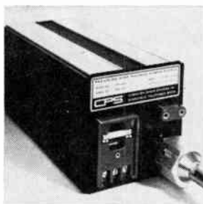
H-v power supply series 1000 is for use in crt display systems, computer output microfilming systems and nuclear instrumentation. It is available in 2 output voltage ranges: 10 to 20 kv, and 20 to 30 kv, with regulation to 0.001% for line or load variations, and a low drift of less than 0.005%/hr. Computer Power Systems Inc., 722 E. Evelyn Ave., Sunnyvale, Calif. 94086. [386]
