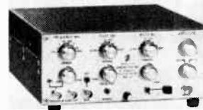
Pulse generator PG-11 provides single or double pulses, pulse pairs, pulse bursts or one-shot output. It operates over a repetition rate range from 10 hz to 20 Mhz in the double pulse mode and to 10 Mhz in the single pulse mode. Rise and fall times are 5 nsec max. at full \pm 15 v output amplitude. Price is $375. Chronetics Inc., 500 Nuber Ave., Mt. Vernon, N. Y. 10550. [367]
