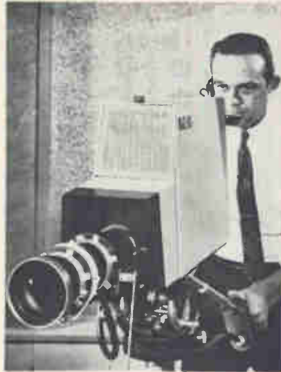
Two down. RCA's new color television camera has one pickup tube instead of the conventional three.
