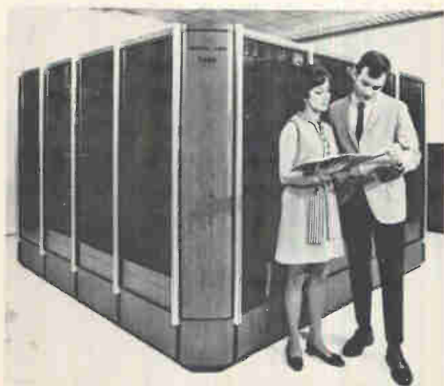
Big and small. Control Data's new computer, the 7600, is big enough for a man to step inside. And it uses tiny (16-mil) hand-wired arrays of toroidal cores in its memory. Despite its use of cores, the machine has a 275-nsec cycle speed.
