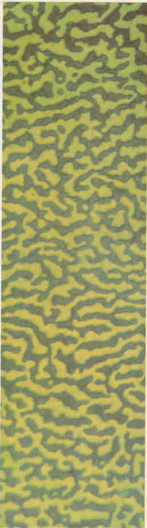
Many small magnets. All the separate magnetic domains are visible under a high-power microscope.
