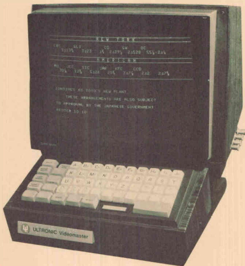
Videomaster stock market display system uses low-cost computer readout CRT to obtain crystal-clear display in a minimum of space.
