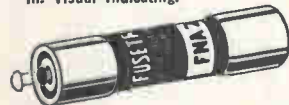
FNA FUSETRON Fuse 13/32 x 1 1/2 in. slow-blowing, Visual-Indicating, Alarm-Activating. (Also useful for protection of small motors, solenoids, transformers in machine tool industry.)
