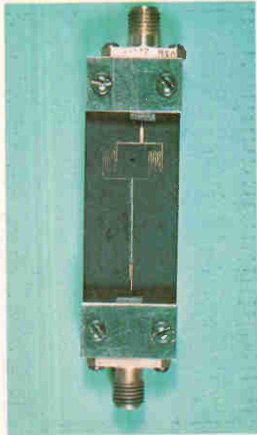
Planar field-displacement isolator. This X-band device uses two nonreciprocal phase shifters that feed a resistively loaded coupled line. Microwave energy is attenuated in one direction but suffers little loss in the other.
