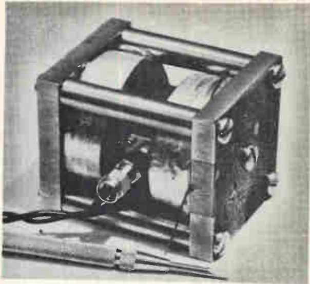
Swept microwave oscillator. Combination of Gunn diode, a yig sphere, and an electromagnet produces at least 50 milliwatts of c-w power from 6 to 12 Ghz.
