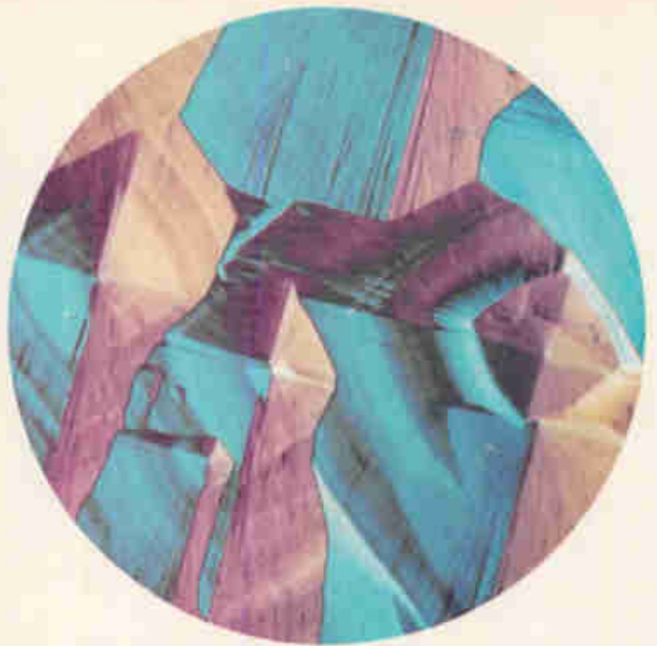
Mountain range. What appears smooth is really a faceted growth of an epitaxial ferrite film when magnified 250 times.
