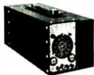
PORTABLE RUBIDIUM ATOMIC CLOCKS 5 \times 10^{-12} /100 sec avg—37 pounds! use Reader Service #318.
