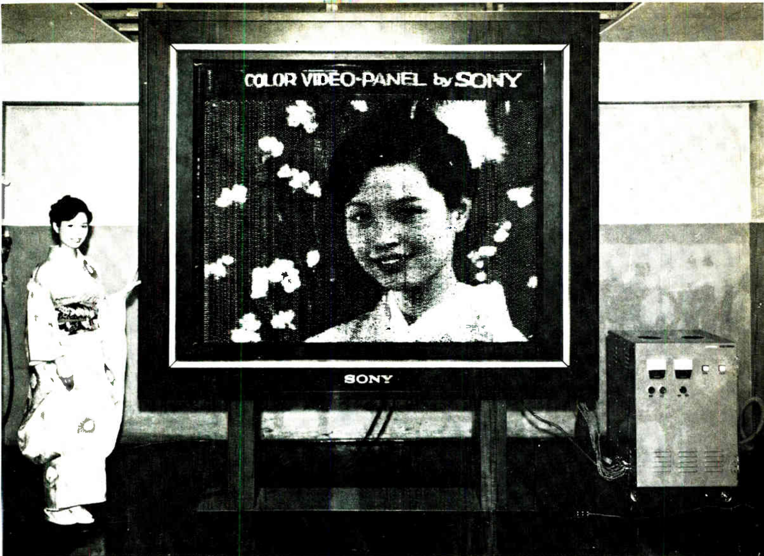
Wide smile. The color video panel, shown with its power supply, right, measures about five by six feet. The message displayed at the top of the screen is generated through a separate channel.
