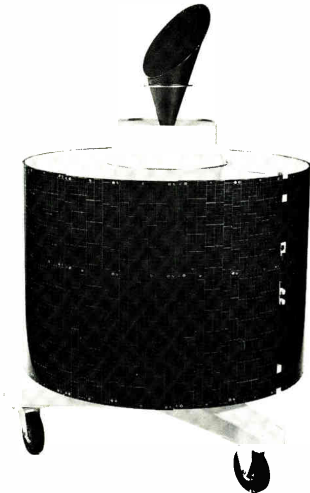
In-line. Mechanically despun antenna shown in mock-up, is mounted atop the Intelsat 3 communications satellite so that they both spin about the same axis.
