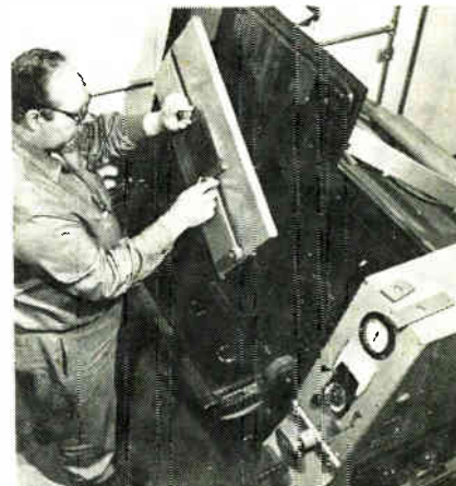
Bathed. Once the artwork is prepared, the steel die is placed in a chemical solution for milling.
