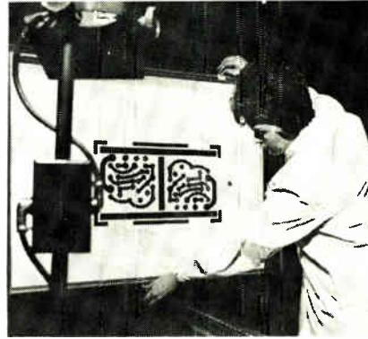
Scaled. Low-cost die stamping process for p-c boards begins with offset reduction of circuit's artwork.
