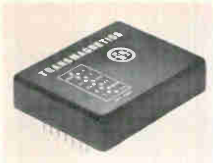
Mod math. Model 450, above, and 749 are designed for p-c board mounting.
