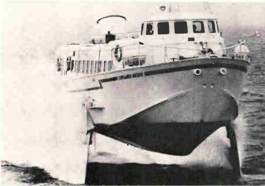
Over seas. The Dolphin-class hydrofoil on which two small dimples below the headlights house transmit and receive horns for sonic height sensor.
