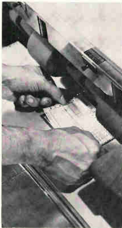
Strike. Bowler inserts scorecard into Brunswick’s computerized automatic scorer, which tallies, prints, and then projects score on a screen.
