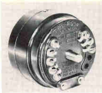
Spinoff. Spinning of shaft produces square waves, and these signals help control cutting and drilling machines.
