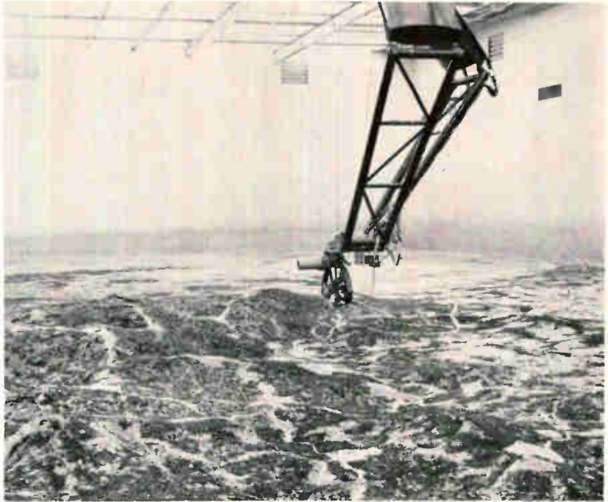
Wide blue yonder. Autonetics makes use of a tv camera transport assembly and terrain model in its study of image-intensifying electronic devices.
