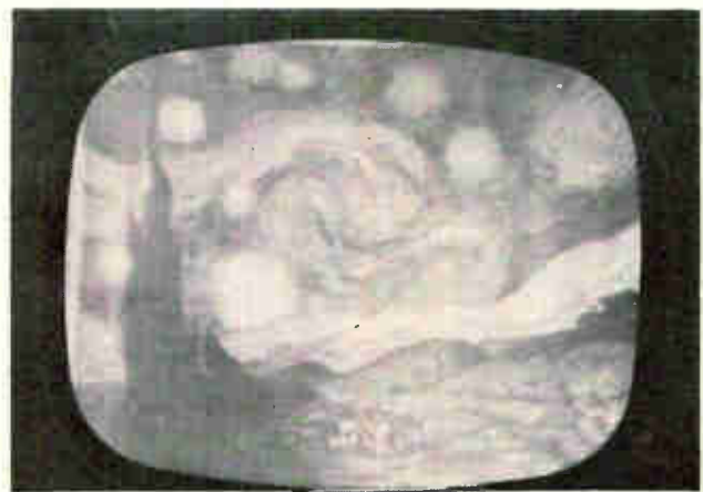
High resolution. The picture at right looks sharper than the one at left but takes no more bandwidth to transmit. The secret is a raster modification developed by two NASA scientists, Edwin H. Hilborn and Lloyd E. Stevenson.
