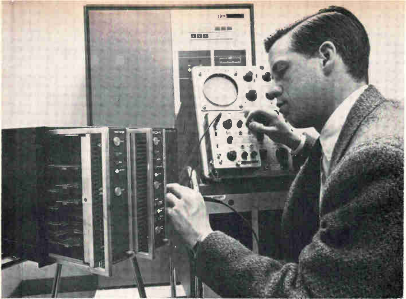
Testing. Author Frey tests Dacor, which is composed of an encoder and decoder. Tall unit at rear is a previous error-correction system made without IC's.
