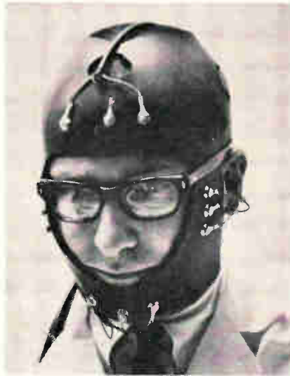
Sensitive. Helmet with electrodes picks up weak voltages transmitted from the brain to jaw muscles. The system cuts a pilot's reaction time.
