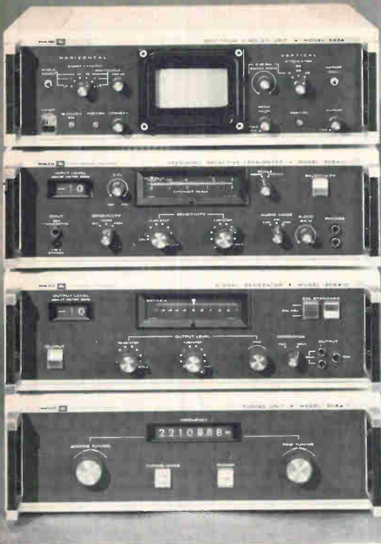
Three 4-kHz channels of L3 carrier multiplex system. Center channel has teletype subcarriers. Model 360A is in 12-kHz sweep width mode, sweeping from 6.780 to 6.792 MHz.
