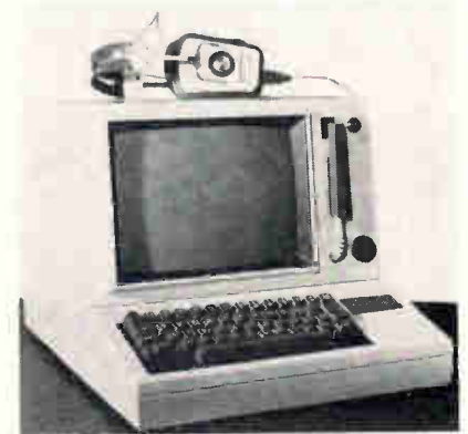
Teacher's pet. The cathode-ray tube of this RCA display terminal for a computer-aided instruction system uses a television-type raster scan.
