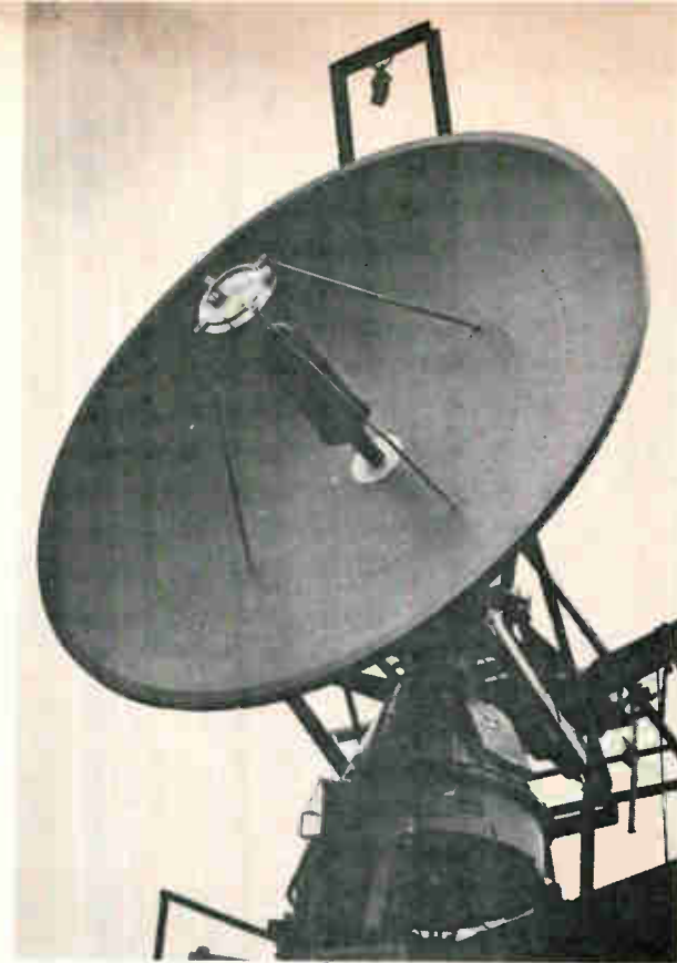
Two in one. Dual-polarized, 10-foot parabolic antenna, built by the Technical Appliance Corp., eliminates the need for second unit in 6 and 11 Ghz microwave service.
