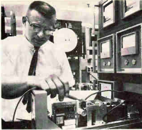
Ounce of prevention. As a result of stepped-up research in the pollution field, more water-quality monitors like this nine-parameter Beckman unit are ready for market.
