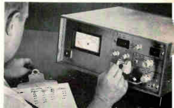
Function plug-in. Module for field-effect-transistor tests fits into unit housing power supplies and readout.
