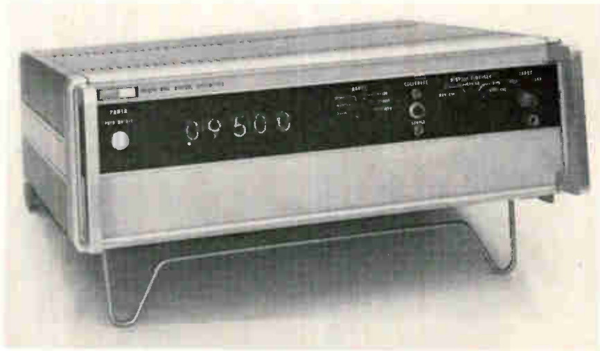
Self-calibrating. Between readings, the a-c digital voltmeter checks itself out. A front-panel lamp indicates when this is taking place.
