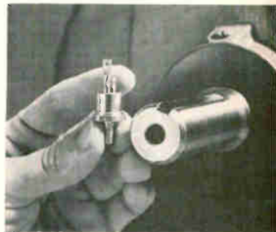
Middleman. Rated at 25 amps, triac fills the gap between low- and high-power solid state a-c controls.
