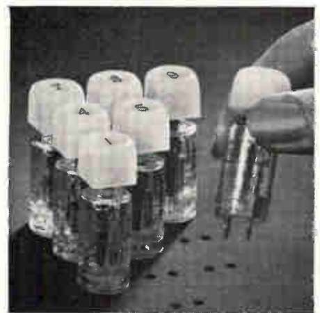
Simple, low-cost mounting. Raytheon switches plug into .125" PC board. Contact pins snap in, firmly lock switch in place for soldering. This permits you to use flow soldering techniques—cut keyboard assembly time and costs.
