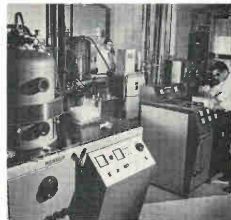
Inside job. Vaporizing apparatus is used to metalize base materials at SGS-Fairchild's Milan research lab.
