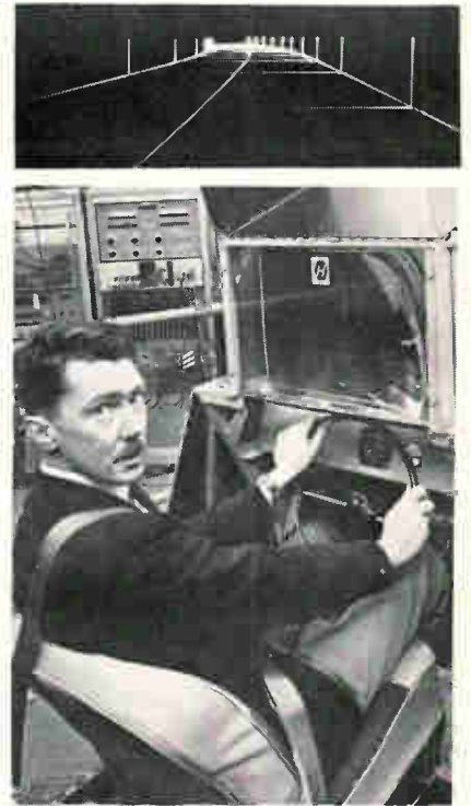
Long look. Driver, seated before a collimating lens, sees unending line of "fence posts" stretching outward to infinity.
