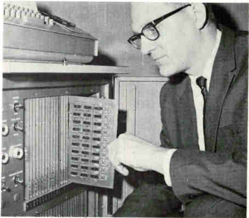
Designer's choice. Chief engineer Kenneth C. Linder selected TTL integrated circuits for, among other reasons, better noise immunity.
