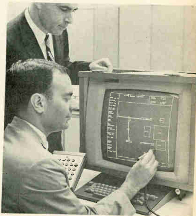
Light-pen operation. Martin Goldberg, author, points light pen at the left edge of a component while co-author Arnold Spitalny looks on.
