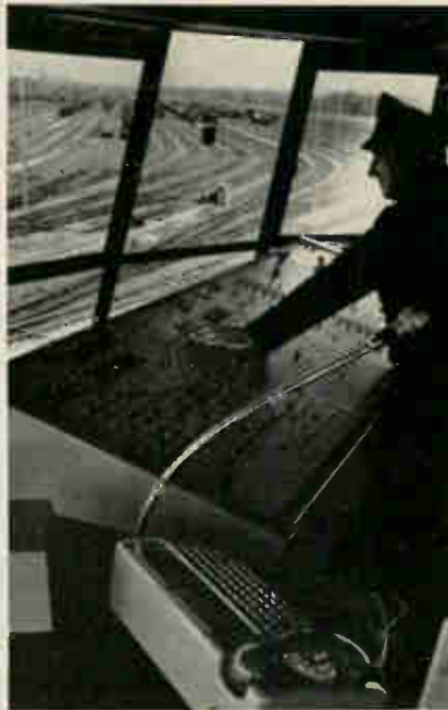
Orders. Computer 45 miles away tells switchman how to assemble trains.
