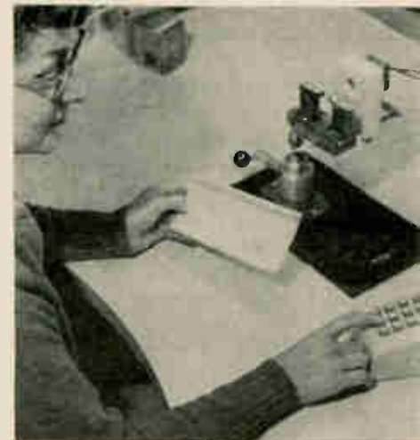
Dialing trouble. Western Electric is computerizing its testing of crystals. Information is entered through a touch-tone dial system.
