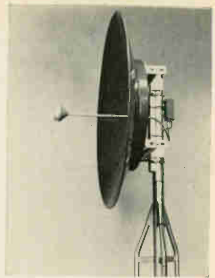
. . . Receiver dish. Receiver converter is also mounted right behind dish.
