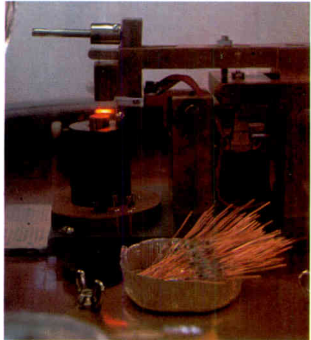
Package sealing. Resistance-heating coil around the switch assembly fuses the glass film to the upper lead and seals the switch.
