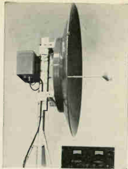
Four-foot dish. Mounted behind antenna is transmitter sending to . . .
