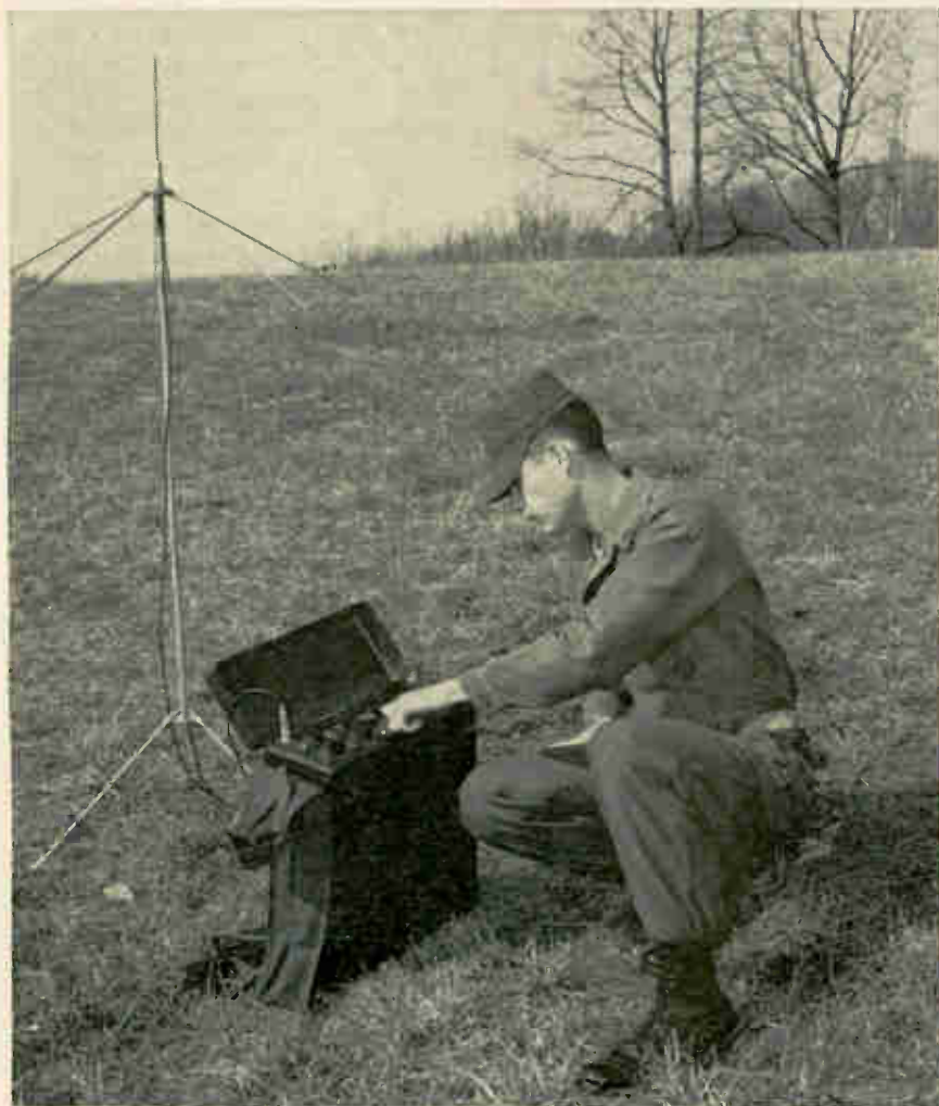
Looking up. The Army is evaluating a manpack system that receives signals from the Navy's Transit satellites, hoping to develop surveying equipment.
