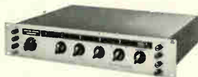
Figure 2. Resolver/Synchro Simulator provides ideal source for receiver testing.
