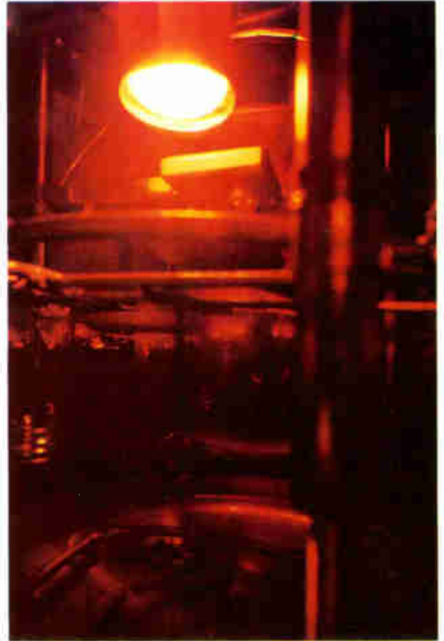
Glass deposition. Substrate heating lamp casts a red glow as the semiconducting glass films are deposited onto the electrodes.
