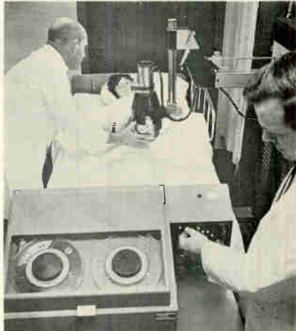
Locating tumors. Radioisotope scanner is positioned over a patient. Unlike ordinary scanners, which produce a paper chart or film image, this system records all data on magnetic tape for computer analysis. A new radiation pattern is recorded every tenth of a second. Computer-processed scans have better resolution than film records. Automatic gain control eliminates the need for extra scans and, perhaps, additional injections.
