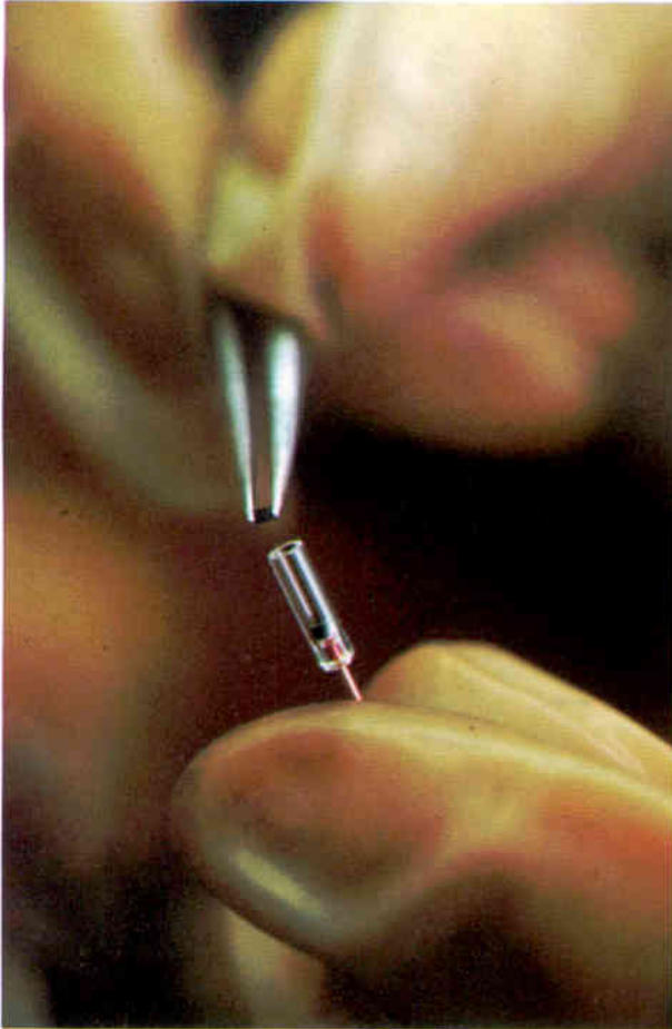
Diode envelope. Since the switches need only two leads, they are sealed in glass diode packages. First sealing step is dropping a coated carbon ball onto the lower diode lead.
