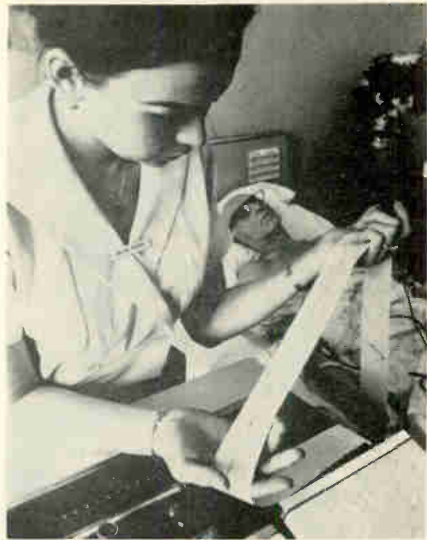
Bedside consultant. Portable electrocardiograph sends EKG signals over a telephone line to a remote computer for analysis. The signals are also recorded in the conventional manner for immediate analysis by a doctor.
