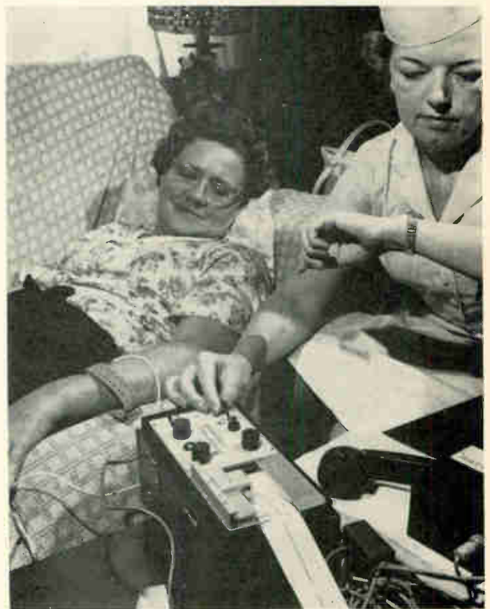
House call. An electrocardiograph records a patient's heart signals in her home and simultaneously transmits them to a computer center for analysis.
