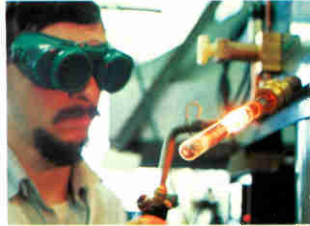
Bomb fusing. Technician prepares bomb by fusing the tube's open end, which is connected to a vacuum line to remove air.
