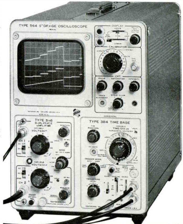
Either half of the split-screen can be used for a stored display, the other half for a nonstored display. (Shown below).
