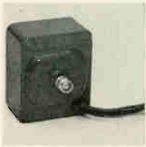
Voltage-tunable magnetron oscillators deliver 500 mw across 1.5 to 3 Ghz. The EM-1321 features flat power output (approximately \pm 1 db). Linear voltage tuning is accomplished by changing the potential of the anode, which has an f-m sensitivity of 1.2 Mhz/v. Dimensions are 2.505 x 3.005 x 2.5 in. Varian Associates, Bomac Division, 8 Salem Rd., Beverly, Mass. [413]
