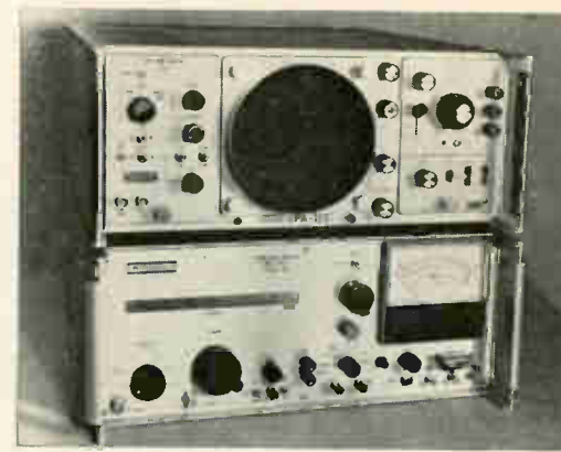
Two-in-one. New receiver to check RFI is two instruments in one: a module that displays spectrums and an analyzer of interference.
