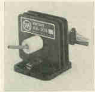
Reflex klystrons, designed for use as pump tubes in parametric amplifiers, operate between 14 and 18 Ghz. The VA-308 delivers between 200 mw and 1 w depending on the choice of beam voltage; the VA-309, from 10 to 300 mw. These powers are available for a 700-Mhz tuning range. Each tube weighs only 4 oz. Varian Associates, 611 Hansen Way, Palo Alto, Calif. [412]
