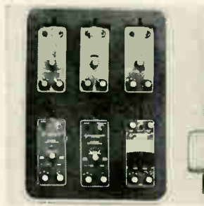
Field-installation checkout of ECM systems is provided by a portable microwave test set. The 693 includes fixed tuned signal generators—at L, S, C, X, and K u bands—and a video amplifier that are operated by built-in rechargeable batteries. Also included are an antenna, detectors, attenuators, and other accessories. Kollmorgen Corp., 347 King St., Northampton, Mass. [415]
