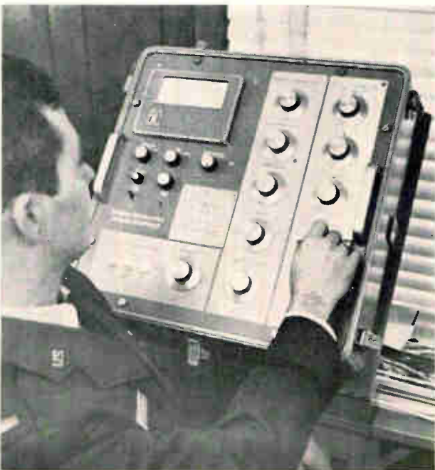
Ground resolution analog computer predicts resolution for a given sensor under expected conditions.
