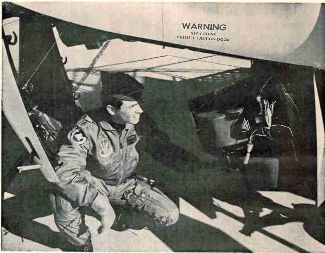
After U-2 was shot down new cameras were developed to come in low, under enemy radar beams. This KA-56A folds up into the sleek RF-4C Phantom and photographs the terrain horizon-to-horizon from as low as 250 feet moving at 600 knots. The camera can process its pictures in flight and has automatic exposure control.
