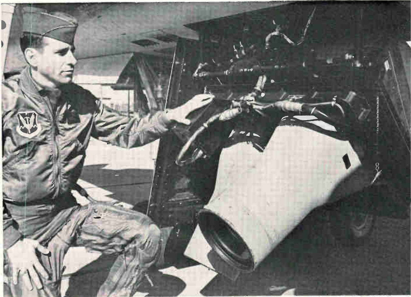
Camera compartment in this RF-101 holds three high- and low-altitude cameras. Black boxes at top contain the electronic switches for camera control.
