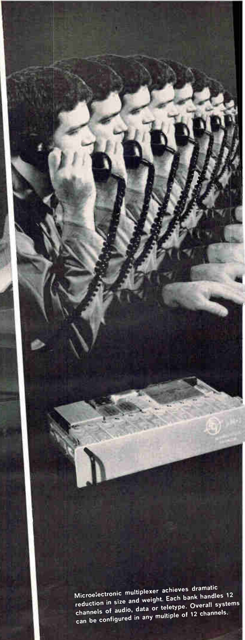
ECI's microelectronic switching systems have automatic solid-state pathfinding, handle voice or data and are compatible with existing system terminals.
