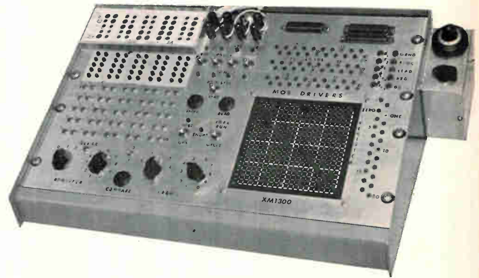
Tilt. Autonetics could build large-scale MOS IC's, but couldn't find a system to test them. So they built their own. Circuits to be tested are mounted at upper left. Test results appear on neon lamp array just below. No news is good news—a lighted lamp means a faulty IC.
