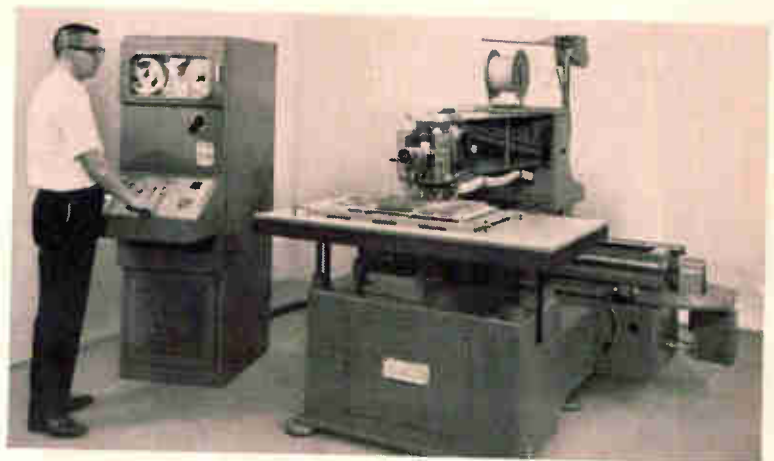
Tape-programmed TERMI-POINT Automatic Wiring Machine routes and fully terminates a 10" lead in less than four seconds.
