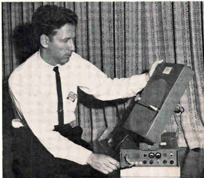
Small wonder—Harold V. Lind, program manager, adjusts antenna elevation of tiny terminal built by Hughes Aircraft.
