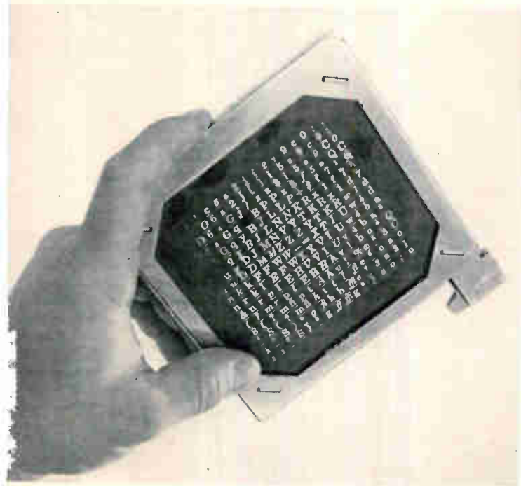
Character grid is a photographic store of 256 type characters. Linotron tube selects one character at a time which is transmitted as a video signal for projection onto crt display.
