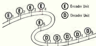
A single pair of wires, or a leased telephone line, can carry the audio signals for a complete control system.
