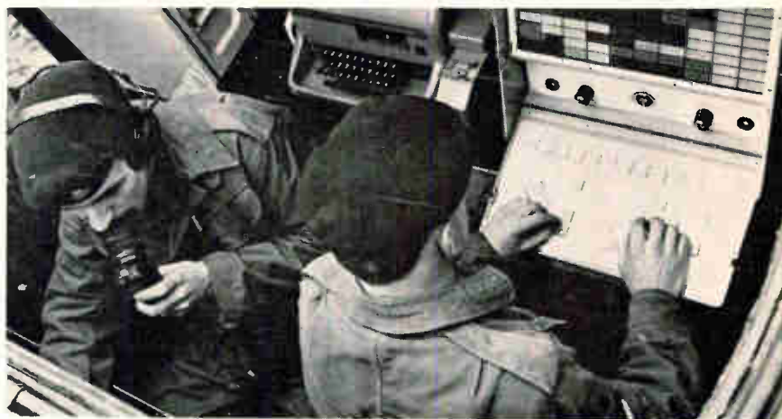
Ready, aim, fire. Officer in armored command-post vehicle relays aiming orders to gunners. Gun positions are calculated by artillery computer from data punched into keyboard.
