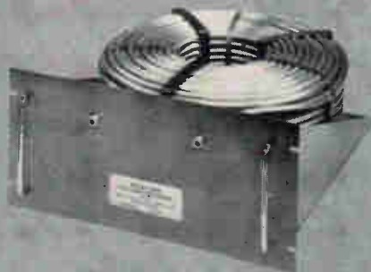
Standard delay line available off-the-shelf for calibration of oscilloscopes, altimeters, radar systems and similar applications. The Foamflex cable unit measures 8 1/2" x 21" x 19" and offers a standard delay of 500 ns, calibrated to ±0.25 ns.
