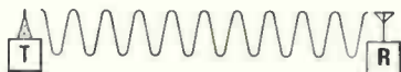
For inaccessible areas or mobile installations, a radio transmitter and receiver system can carry the signals.
