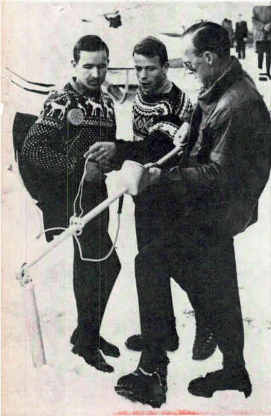
Alpine lifesaver. Sensor dangling from aluminum pole can spot skier buried under 10 feet of snow—if he's wearing tiny permanent magnet. Electronics pack carried on rescuer's back weighs just 7 pounds.
