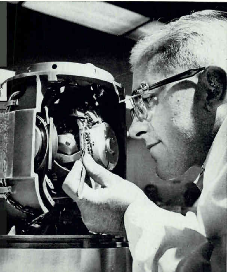
Sperry's SGN-10 is the first inertial guidance system for airliners. Technician checks the gyro reference unit for flaws.
