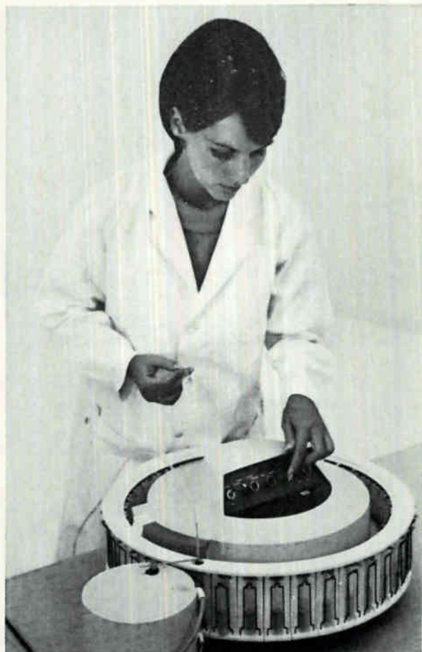
Automatic liquid sampling device provides test results in computer format for Technicon's Autoanalyzer. The reader in the system is built by IBM.
