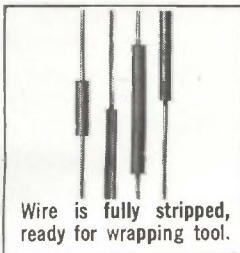
Remaining insulation can be short as 1/2".
