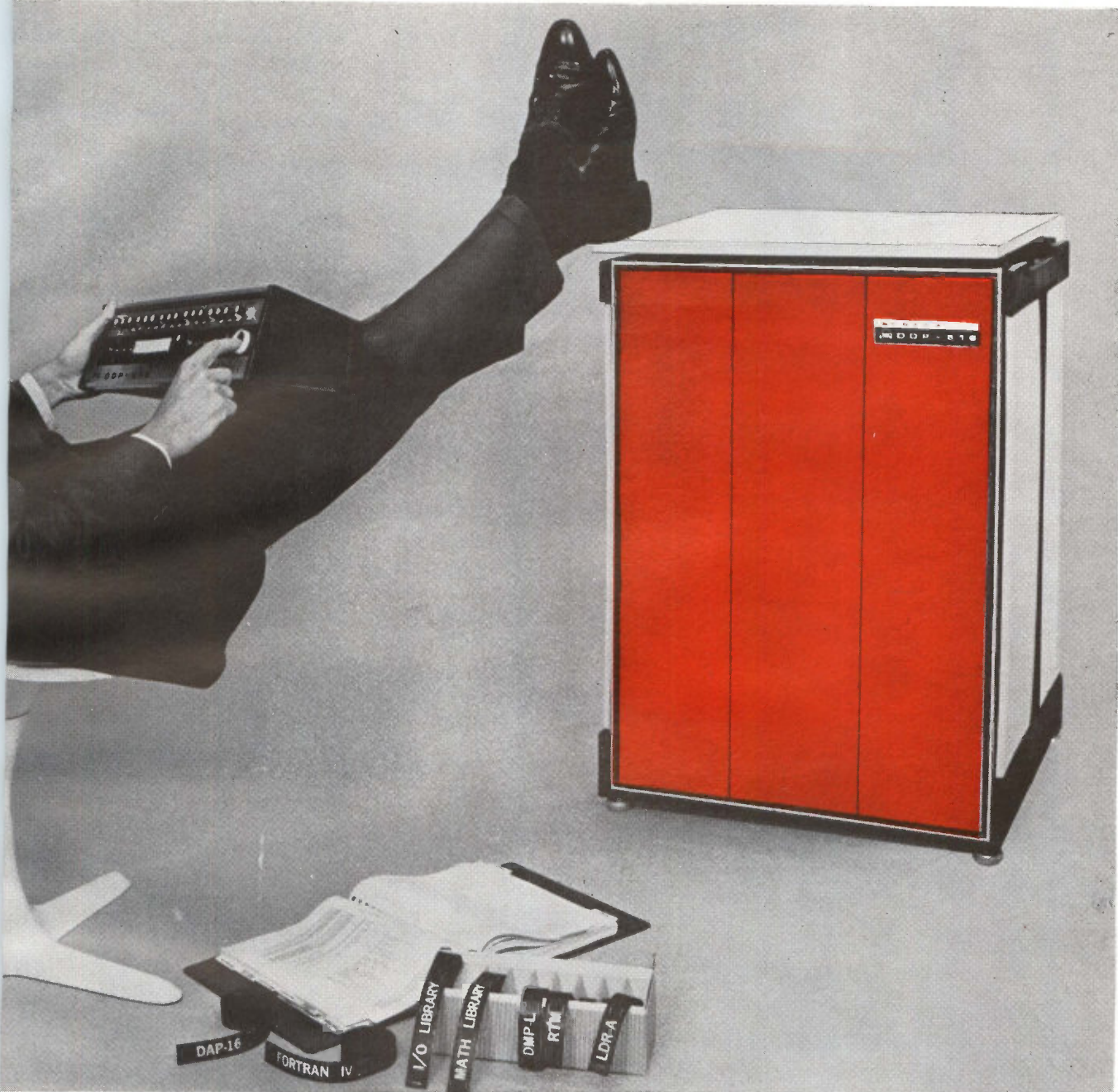
Above: DDP-516 with 16K I/C core memory.
