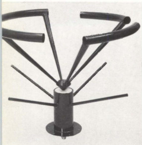
Pop art antenna, to be mounted on an aircraft's fuselage, was specifically designed to operate with satellites.
