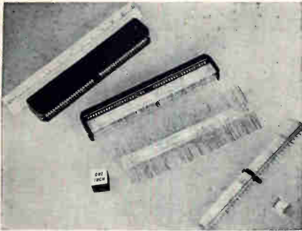
Earlier form of welded logic module has welded cross-wire matrixes that interconnect discrete components. The matrixes are made on numerically controlled machines.
