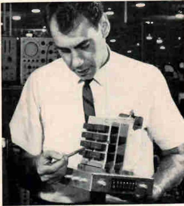
Digital modules make up the exciter circuit which measures 6 x 6 x 8 inches. The circuit has a frequency response extending to 300 kilohertz.
