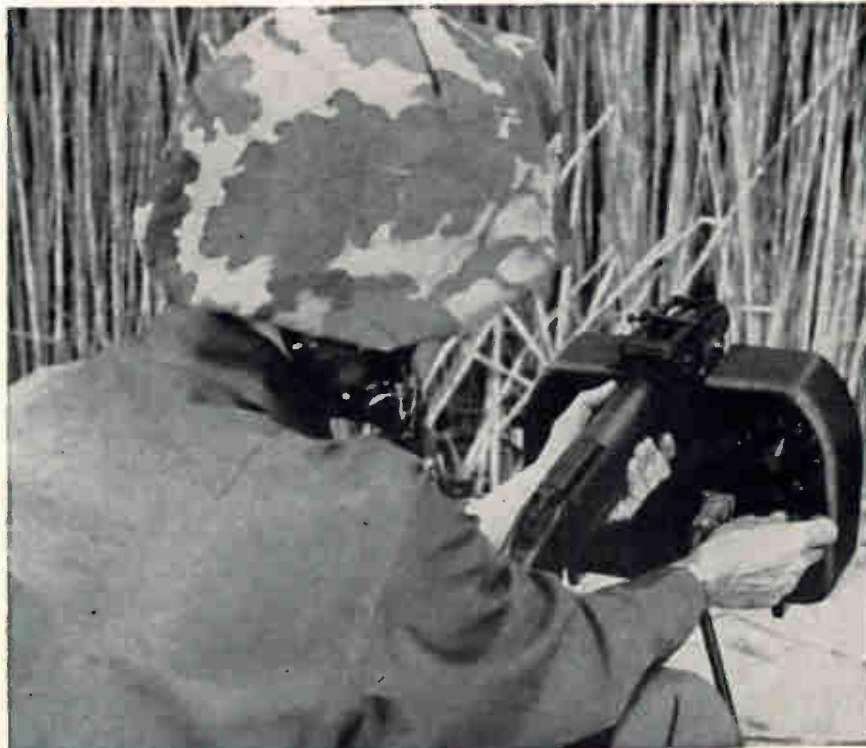
Two-pound radar developed by the Radio Corp. of America. Unit can detect a man 300 meters away and a vehicle at 1,000 meters. A model with far-better range is being developed.
