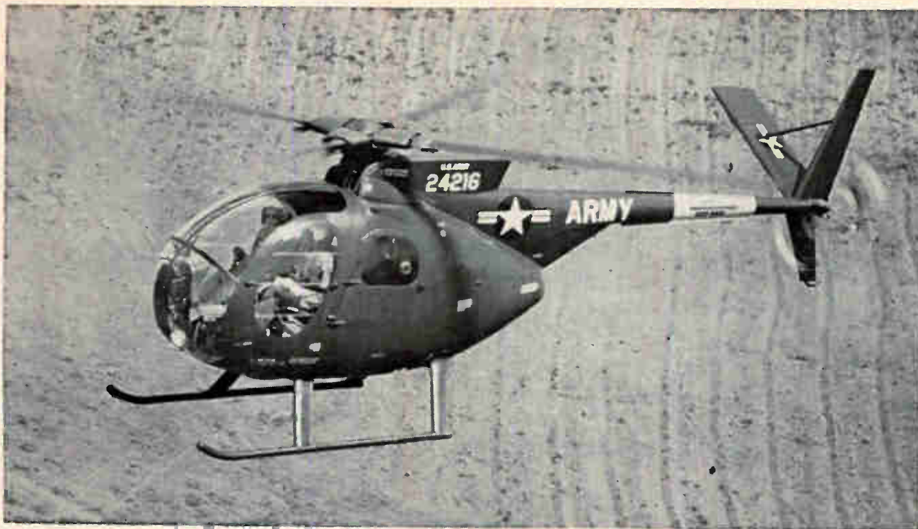
Light observation helicopter, packed with new communications equipment, will spot enemy artillery and troop movements. It will replace the fixed-wing planes now in use.
