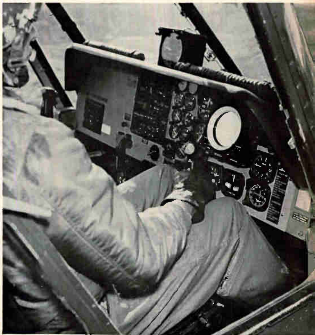
Station-keeping system , developed by the Sierra division of the Philco Corp. The scope in the control panel is the system's plan position indicator.
