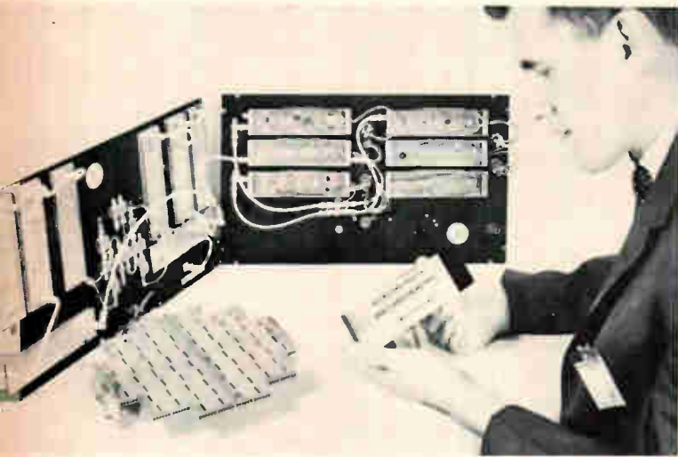
Doppler radar system, built for the Air Force, demonstrated that it was practical to mix Mirt and Lava chips in breadboarding prototype equipment. Breadboarded system is in background. Bill List holds actual-size model of final equipment.
