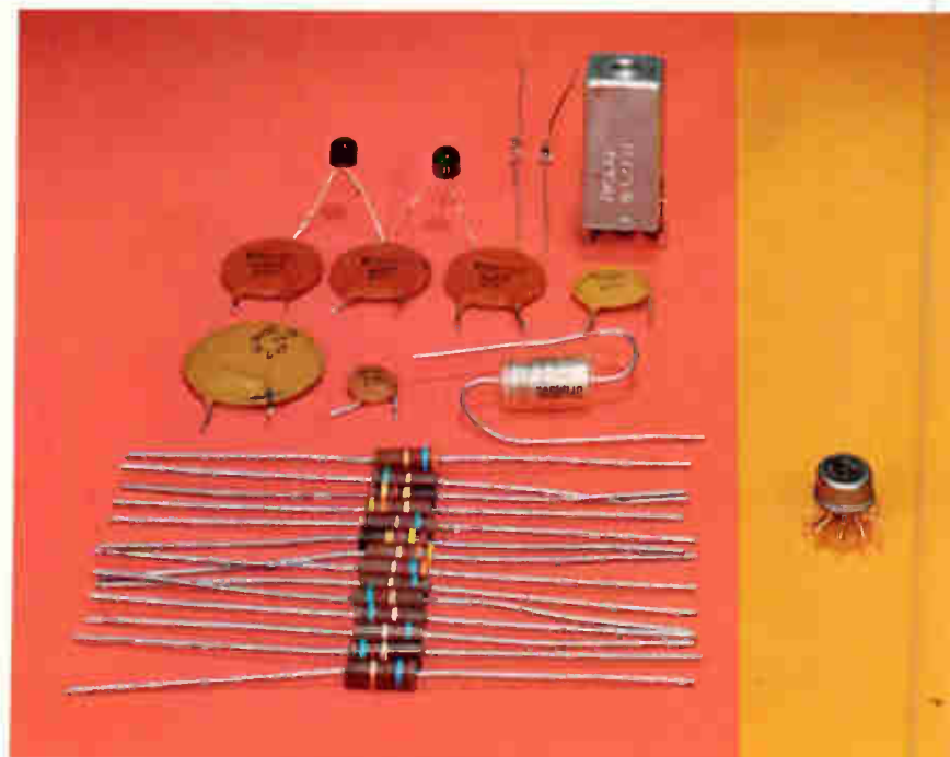
Integrated circuit replaces the discrete components shown. Eliminated are 2 transistors, 2 diodes, an interstage transformer, 14 resistors and 7 capacitors.
