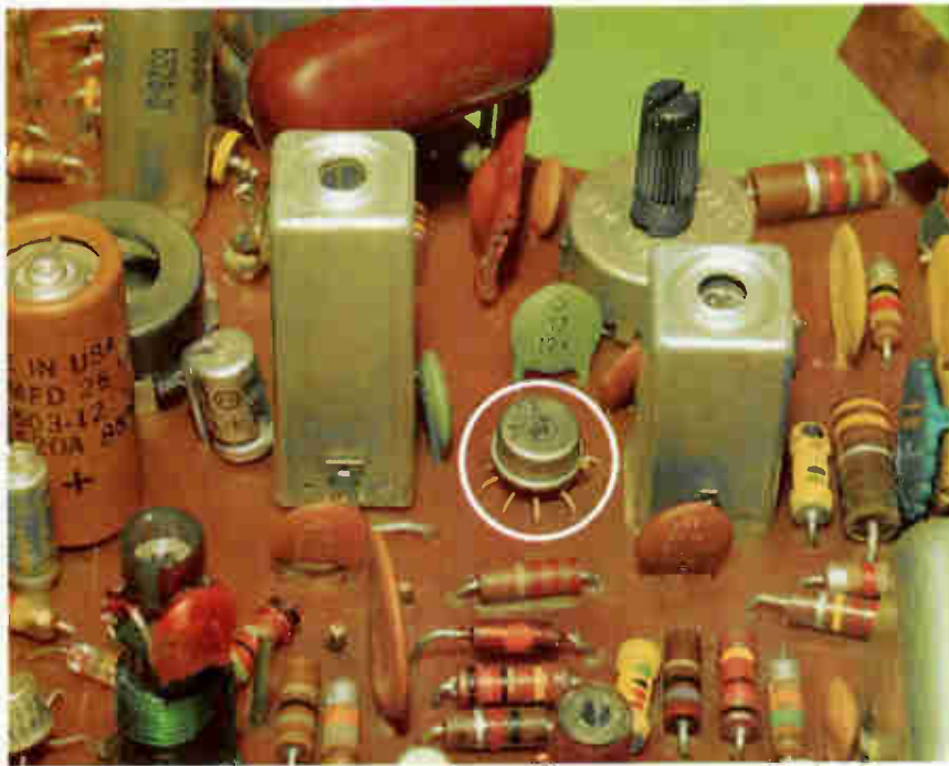
Integrated circuit in a production-line tv receiver manufactured by the Radio Corp. of America. Circle denotes the IC. Large cans are transformers.
