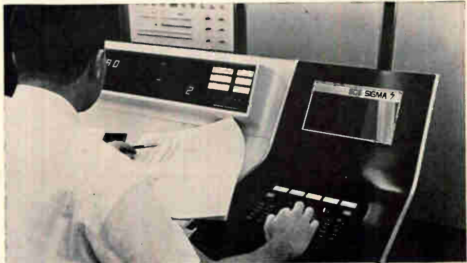
Programmer operates a keyboard to control time-sharing computer system of the Sigma 7.
