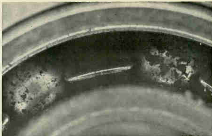
Heat damage to capstan bearing of a tape recorder subjected to 145°C during three 36-hour heat cycles.
