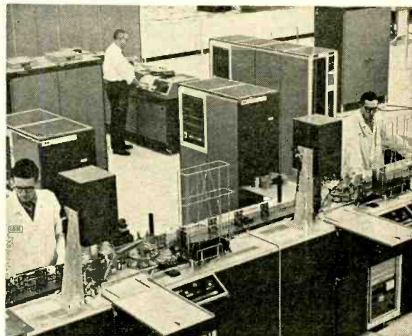
After a computer-controlled assembly machine plugs logic circuits into the cards, more than 2,000 wiring and logic tests are made on each card by this machine, whose control computer is programmed by the logic-design computer.
