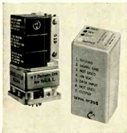
Series 300 voltage-controlled oscillator is assembled from reliable, dice-size electronic building blocks to give versatility in performance (left). Test point and potentiometer adjustments for output, deviation and center frequency are accessible through the cover (right).
