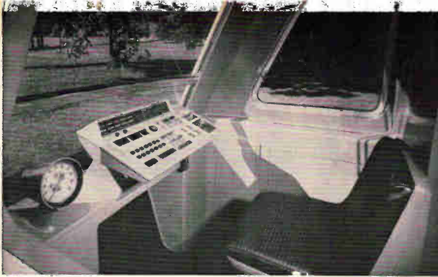
Interior of detachable pod at front of BARTD train. One sits here to take control in case of emergency. With the control panel the crewman monitors the electronic control equipment on board; through the large front window he watches for fallen boulders and other track obstructions. He won't have to watch for people or for stalled cars; the track is completely fenced and there will be no grade crossings.
