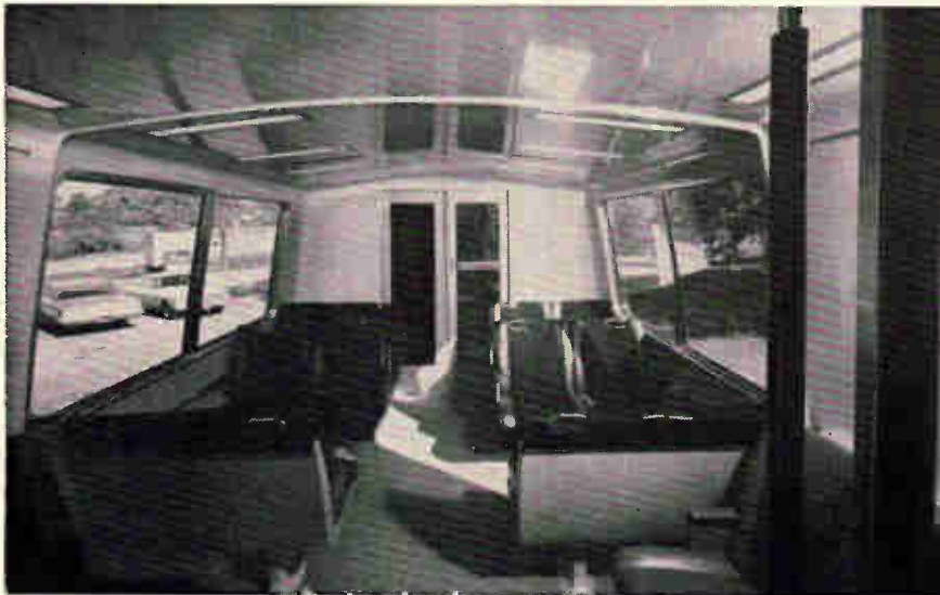
Interior of passenger section of BARTD rapid-transit car. The upholstered seats—charcoal and brown in this prototype model—are 22 inches wide, compared with the usual 17 or 18 inches for bus seats. The decor includes beige carpeting and vinyl wood-grain paneling. The prototype car is now on display near San Francisco, and BARTD officials have invited the public to inspect it and make suggestions.
