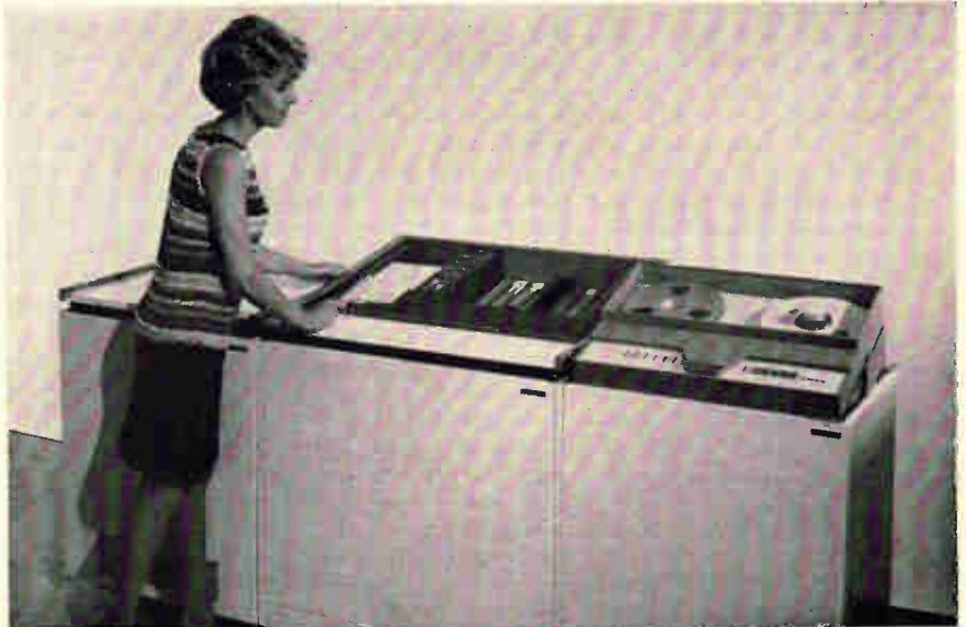
The Ampex CTS-2000 transfers computer data from 2,000 tab cards to magnetic tape in one minute.
