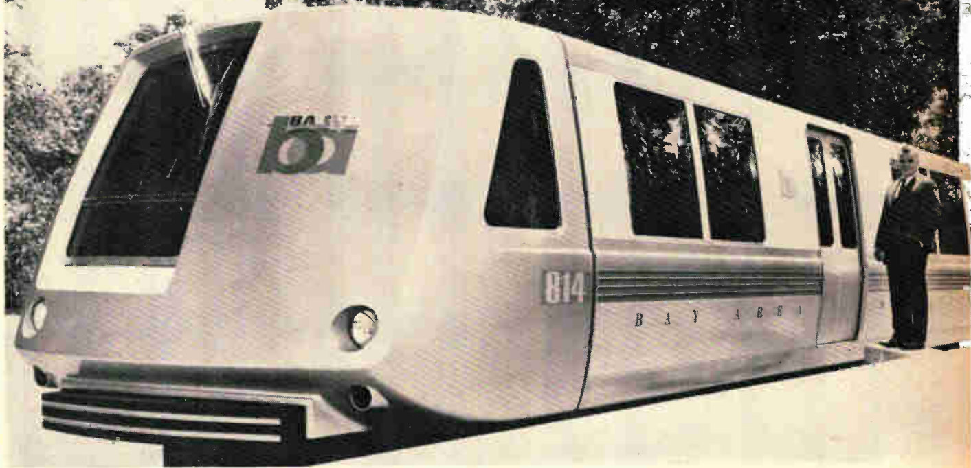
Prototype of rapid-transit car for the BARTD system. It is 72 feet long, air-conditioned, and carries 70 riders who can look out through tinted windows as they relax in upholstered comfort. The car runs on a wide-gauge 5½-ft. track (standard gauge is 4 ft. 8½ inches) for greater stability and a smoother ride. The detachable front section, or pod, carries all the electronic equipment and the one crewman aboard the train. The exact specifications of the pod will depend on the control system chosen after the test period on the Mt. Diablo track.
