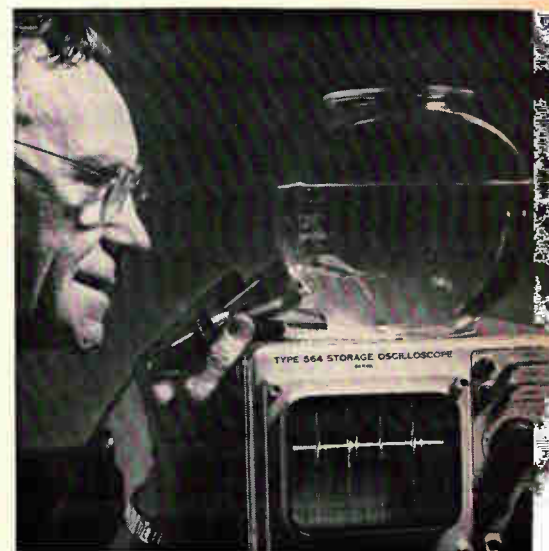
Gill movements of a goldfish are monitored by Richards using his ultrasonic instrument.
