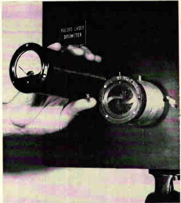
Front view of dosimeter shows lens with scribed marks for lens openings coming between those normally used in photography. Hand-held device is a standard light source used for calibration.
