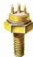
New RCA "Overlay" Transistor. In an area smaller than the head of a pin, this unique device contains 156 microscopic transistor junctions connected in parallel for maximum power amplification at extremely high frequencies.
