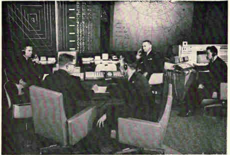
Operators of large-screen display can request new maps, additions to maps, and a variety of information listed in tabular form along-side the map.
