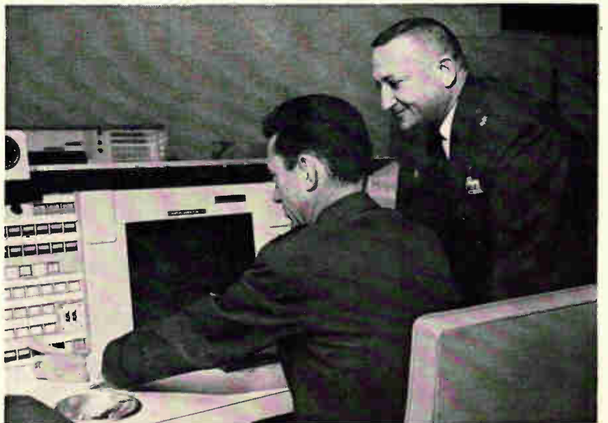
Display console converts digital and video information into figures, symbols and television images on this cathode ray tube.
