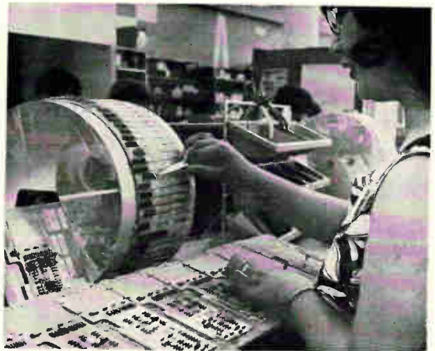
As wheel revolves, the assembler picks up a component and puts it in the circuit board in numbered sequence.
