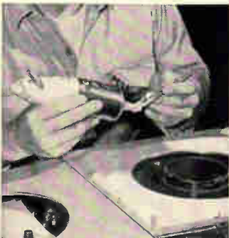
5. RTV laminates layers of mica sheeting and plates in production of plate condensers. Results: improved operational reliability, assembly time cut from 24 hours to 20 minutes.
