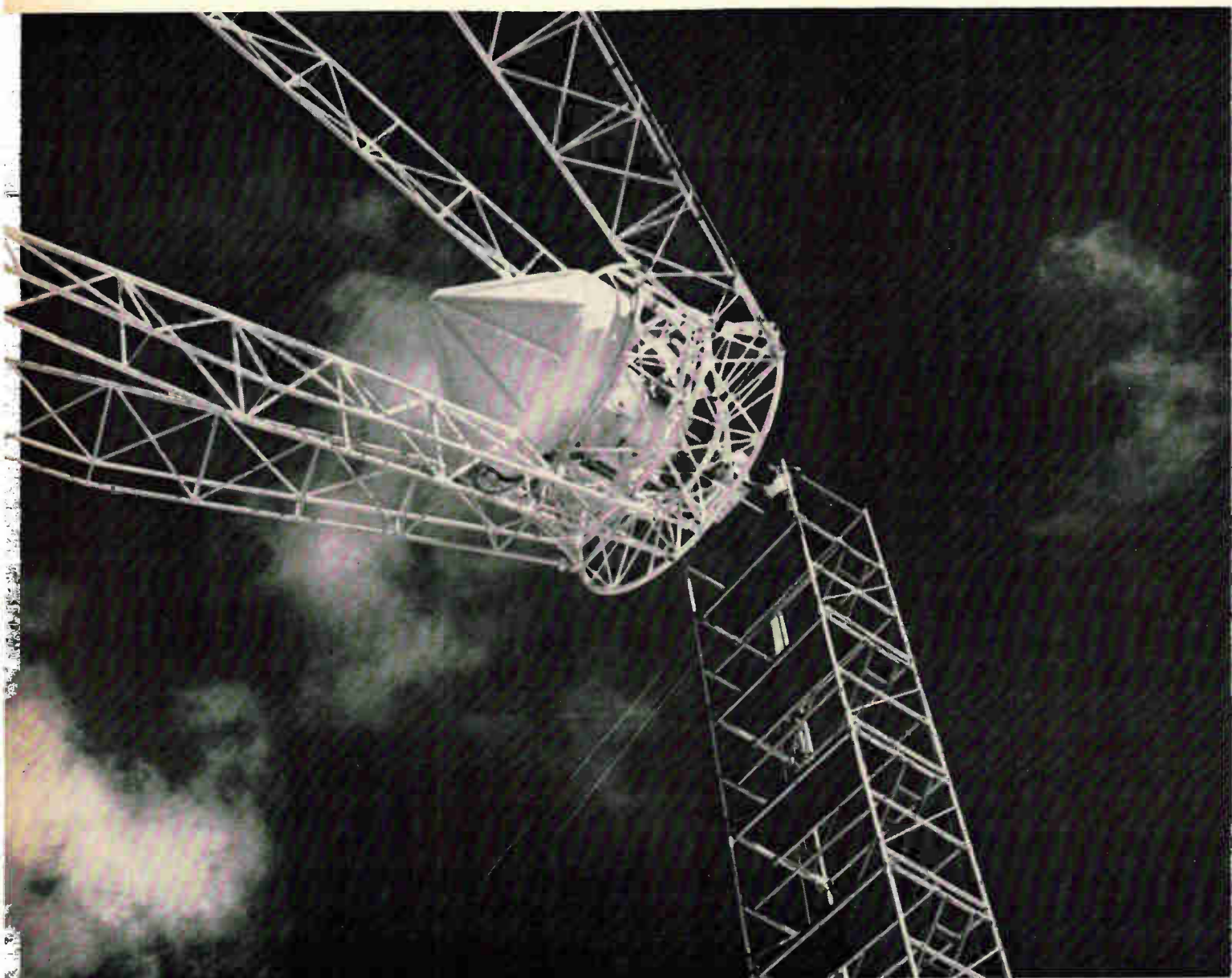
Dual conical spiral feed on the TAA-2 telemetry antenna covers the 130 Mc to 2,300 Mc range.
