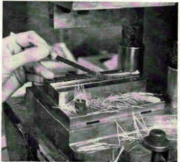
Adhesive tape lifts a row of 50 components out of the press after the press has cut and formed the leads.
