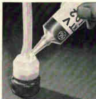
3. RTV seals AN connectors, terminals and wire harness joints and other flexible parts. It will absorb shock and vibration, eliminating the fatigue failure of connections.
