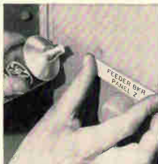
6. RTV eliminates need for screws and drilling when used to affix name plates and decorative emblems on any surface. Results: no unsightly rust drainage; plates stay put indefinitely, but can be cut loose when desired.
