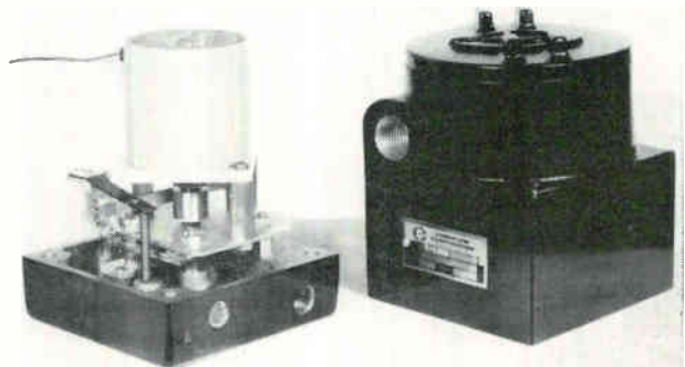
Digital-pneumatic transducer with its cover removed. The stepping motor changes digital signals from the control computer into pneumatic signals of 3 to 15 pounds per square inch by controlling an air nozzle.
